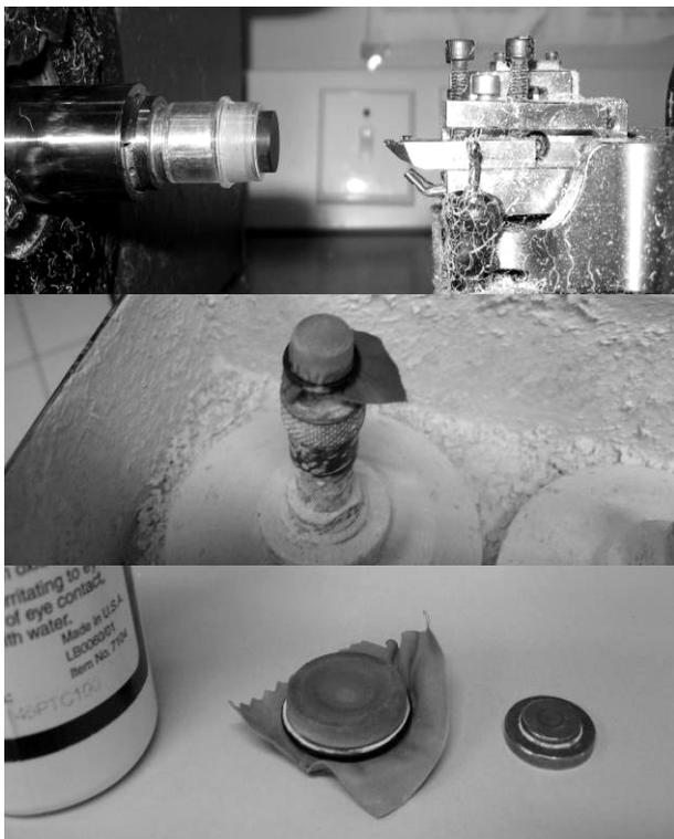
Figure 2. Stages of RGP CL manufacturing process – diamond turning and polishing
