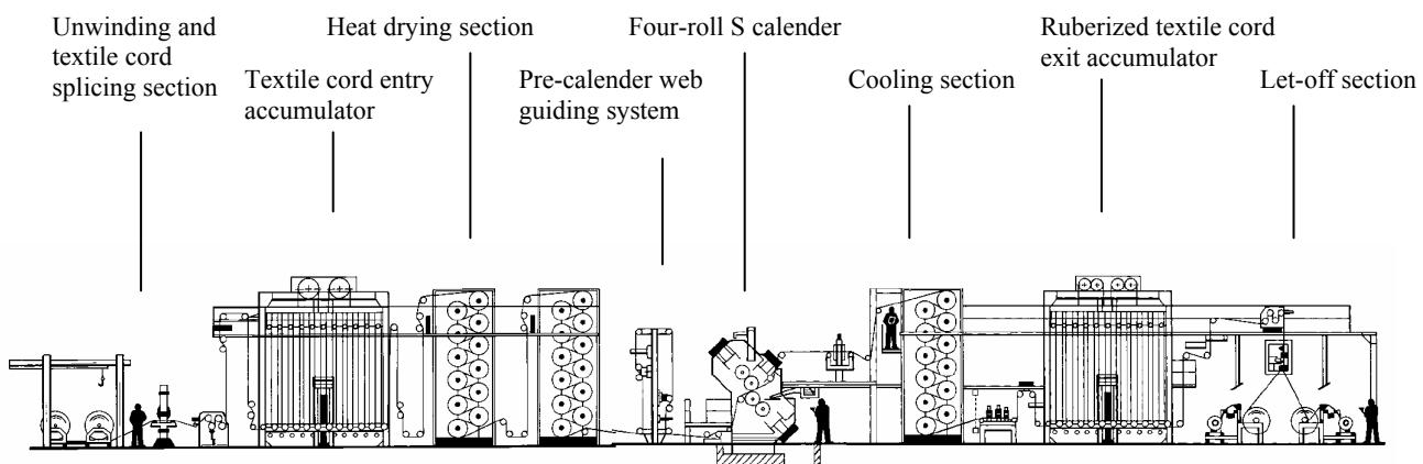
**Figure 2. Typical lay-out of calendering line for textile cord**
