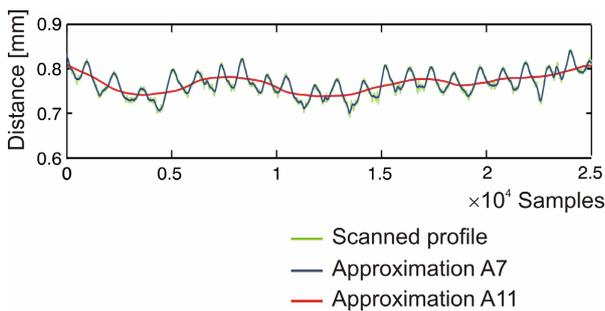
Figure 9: Comparative review of RCS bottom profile (Fig. 6b) and its DWT approximations A11 and A7
