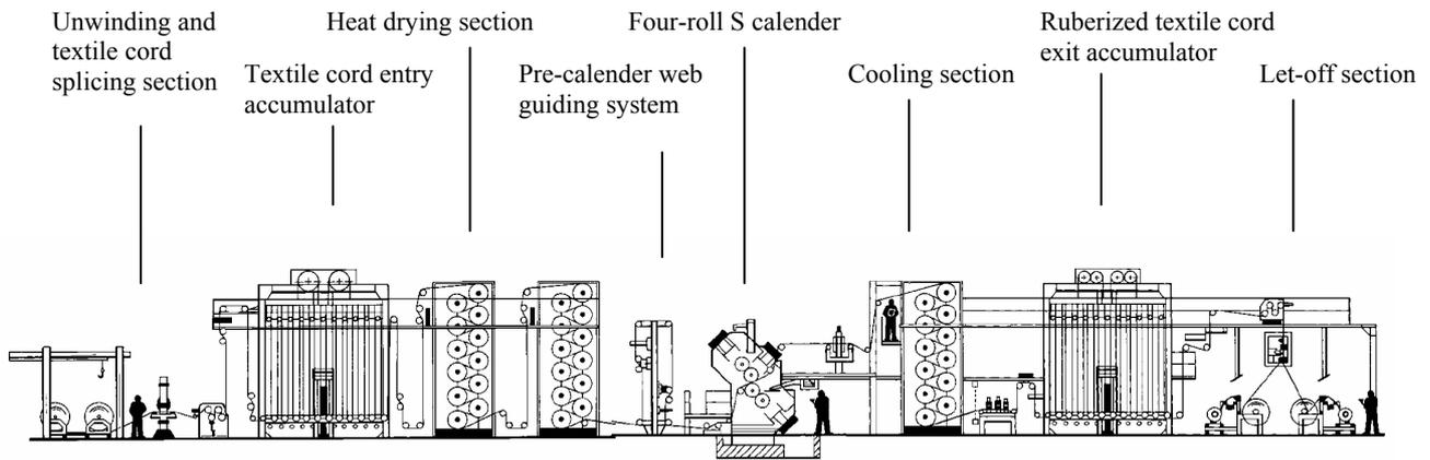
**Figure 2. Typical lay-out of calendaring line for textile cord**
