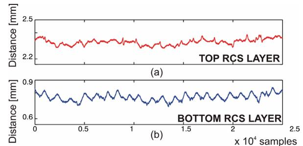
**Figure 6. Parts of scanned profiles of: (a) top and (b) bottom RCS layer**
