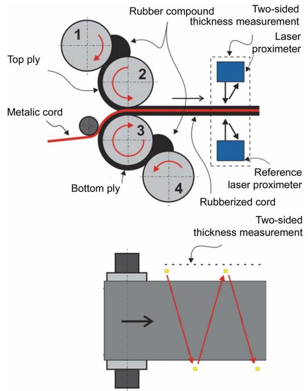
**Figure 4. Cross-section of 4 roll calender in S configuration and layout of a post-calender sensory system**
