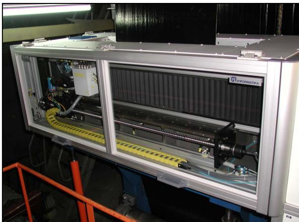
**Figure 5. Prototype of measuring station designed for post-calender thickness measurement of rubberized steel cord (the system was installed in Belshina tiremaking company, Belarus); Measuring module (up) and complete measuring station (down)**
