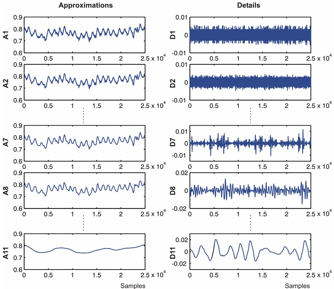
Figure 8. DWT decomposition of the signal given in Figure 6b – levels 1, 2, 7 and 11 using db4 wavelet
