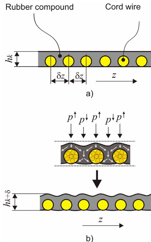
**Figure 3. RCS cross-section profile: (a) ideal and (b) real**
