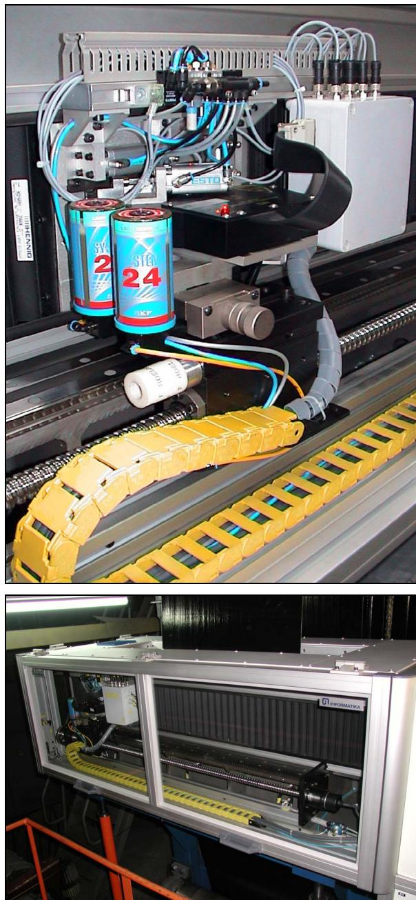
**Figure 5. Prototype of measuring station designed for post-calender thickness measurement of rubberized steel cord (the system was installed in Belshina tiremaking company, Belarus); Measuring module (up) and complete measuring station (down)**
