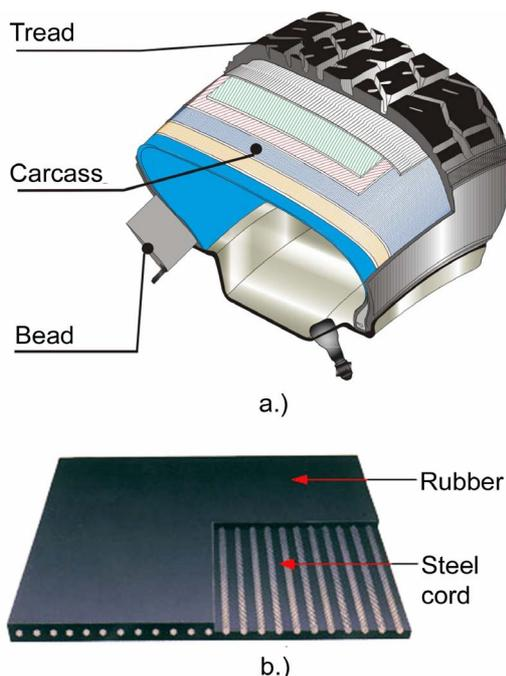
**Figure 1. (a) tire cross-section and (b) rubberized cord sheet**
