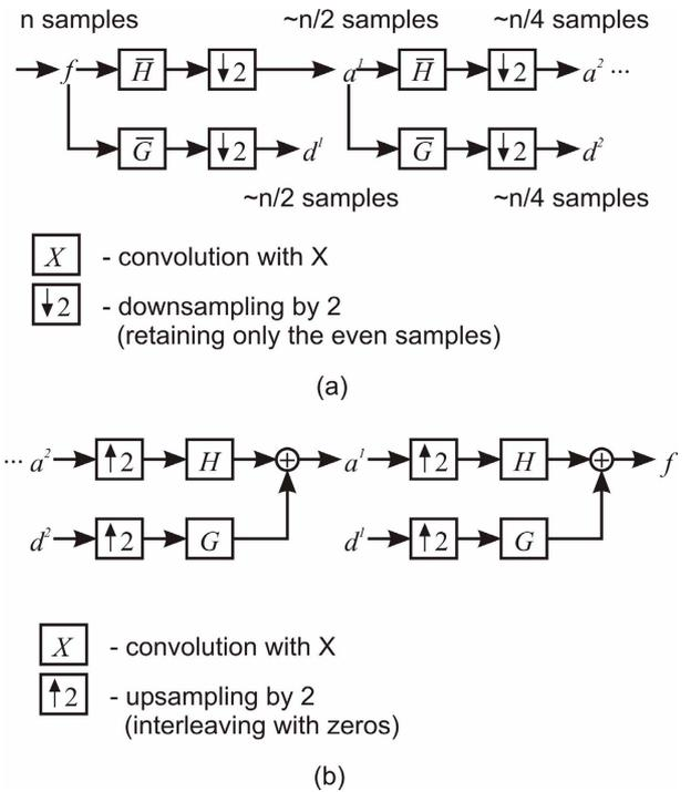
**Figure 7. Subband filtering scheme for: (a) direct DWT and (b) inverse DWT**
