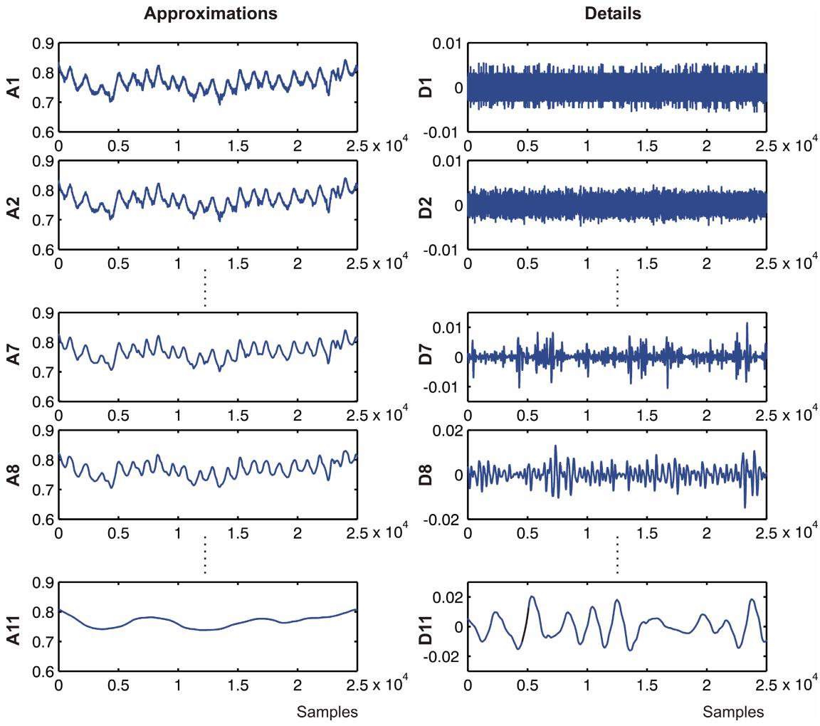
**Figure 8. DWT decomposition of the signal given in Figure 6b – levels 1, 2, 7 and 11 using db4 wavelet**
