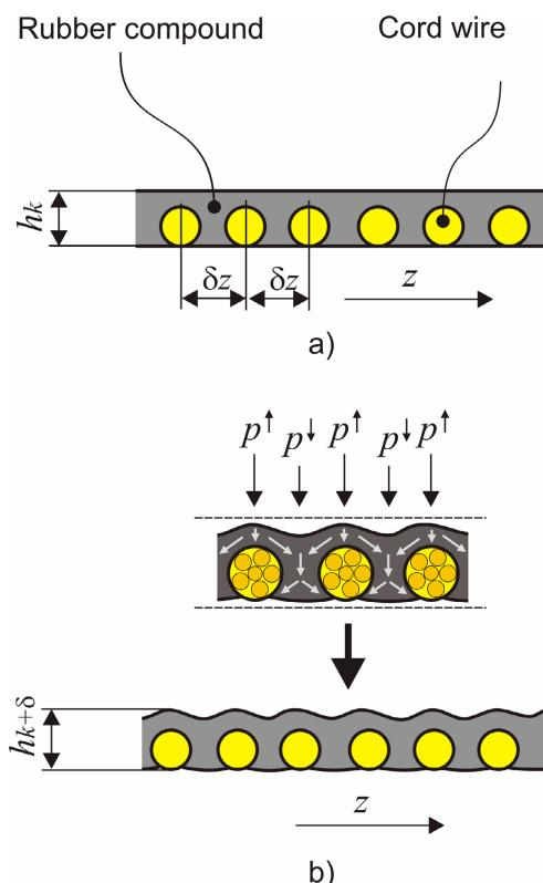
**Figure 3. RCS cross-section profile: (a) ideal and (b) real**
