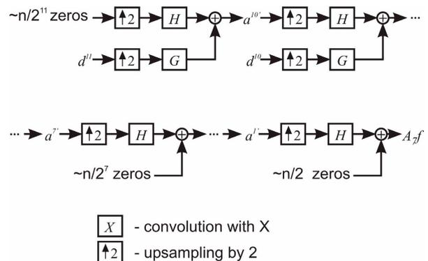
Figure 10. Filtering scheme for extraction of texture
