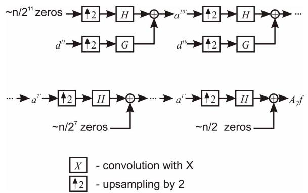
**Figure 10. Filtering scheme for extraction of texture**
