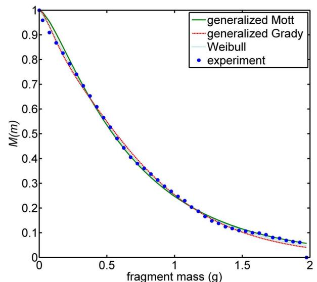
**Figure 2. Relative cumulative fragment mass distribution: comparison of the experimental data (projectile 1 from [19]) and the generalized Mott, the generalized Grady and the Weibull distribution**
