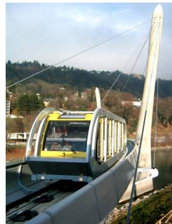
Figure 10. Carriage of the Hungerburg funicular railway [5]
