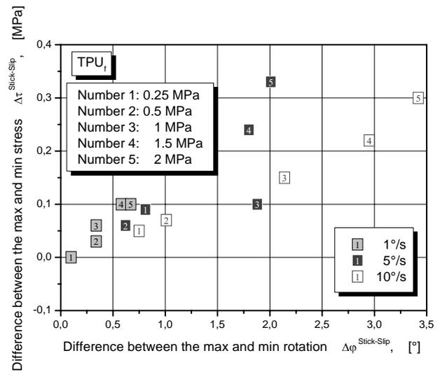
Figure 6. Diagram of the stick-slip deltas in connection to the load and velocity for TPU<sub>f</sub>
