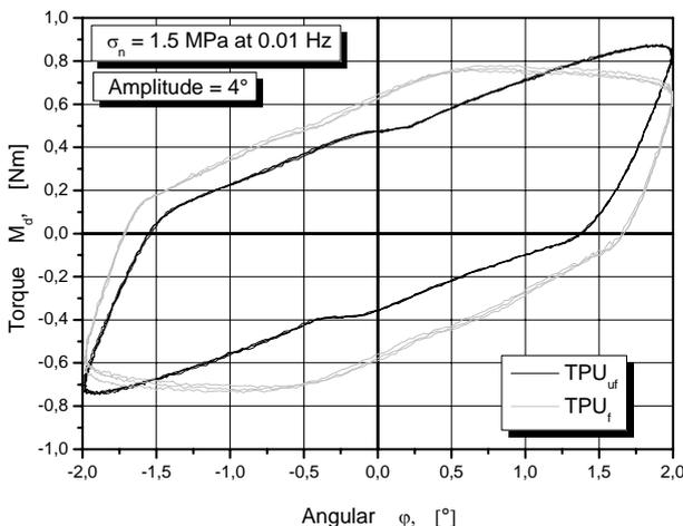
**Figure 9. Difference between TPU<sub>f</sub> and TPU<sub>uf</sub> for high amplitudes**
