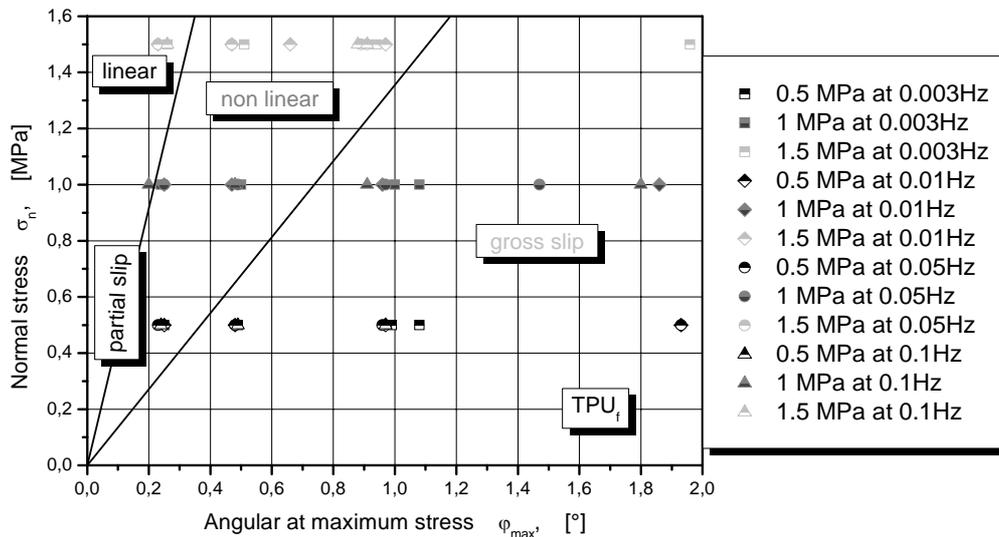
**Figure 8. Running condition stick-slip map for TPU<sub>f</sub>**
