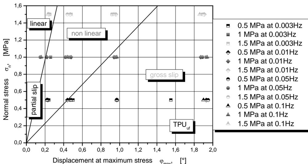
Figure 7. Running condition stick-slip map for TPU<sub>uf</sub>
