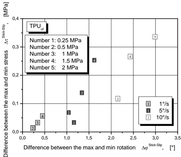
Figure 5. Diagram of the stick-slip deltas in connection to the load and velocity for TPU<sub>uf</sub>
