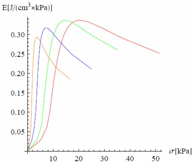
Figure 8. Effectiveness diagram for compression – different specimens and various foam densities
