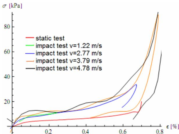
Figure 15. Stress – strain diagram for dynamic and static tests, specimen 10 (red line is a static test curve, other curves are for dynamic tests with four impact velocities approx. from 1 to 5 m/s)
