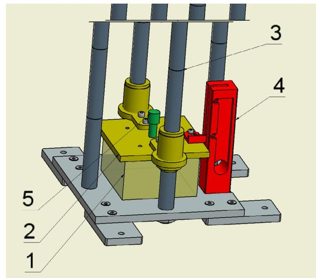
1 – foam specimen; 2 – impactor; 3 – impactor guides; 4 – velocity measure device; 5 – accelerometer
