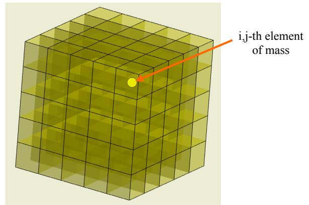
Figure 9. Specimen divided into  $i \times j$  elements
