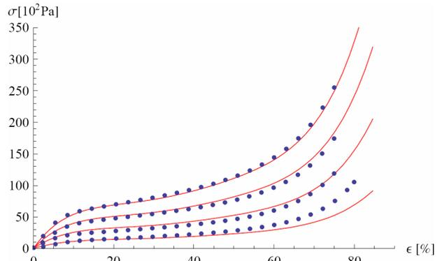
Figure 6. Compression curves for different specimens (continuous line is interpolation function and dark points are experimental results)
