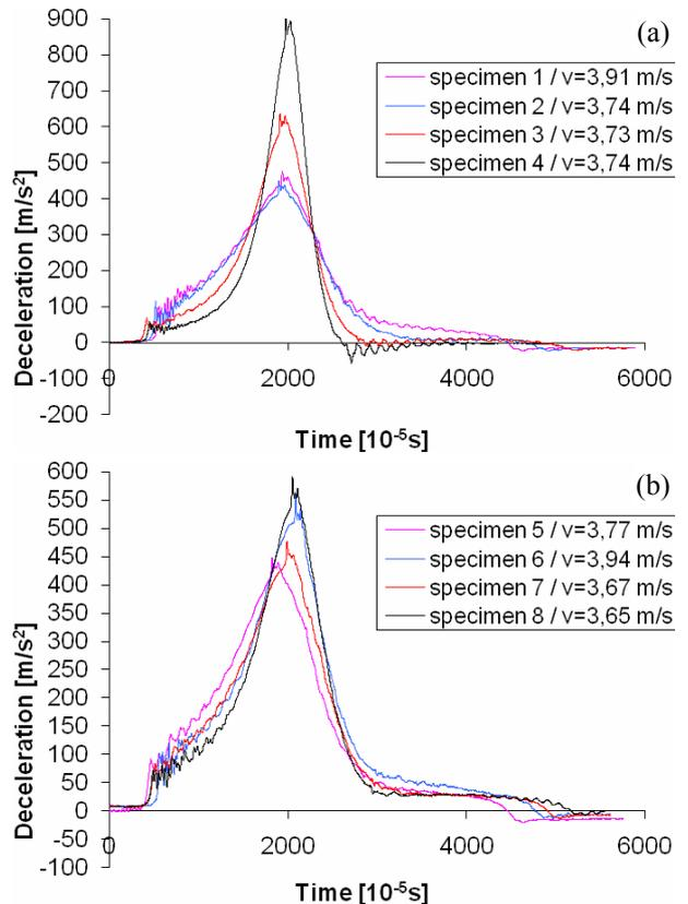
Figure 14. Deceleration vs time for impact velocities about 3.7 m/s: (a) results for specimens of the same densities and various components proportions and (b) results for specimens of the same components proportions and different densities
