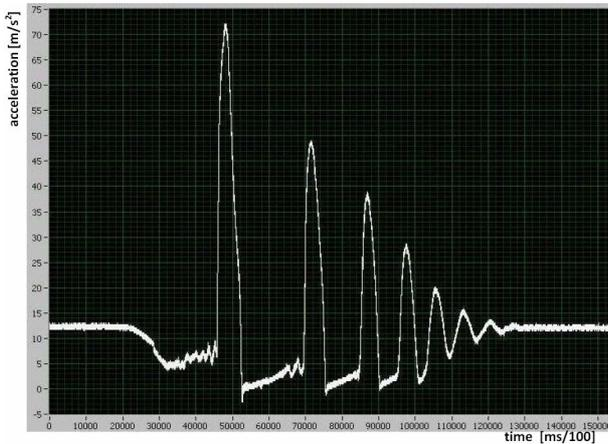
Figure 11. Impact record – deceleration [ $\text{m/s}^2$ ] vs time [ms]
