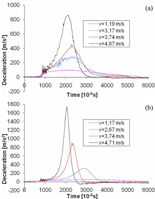
Figure 12. Deceleration vs time for various impact velocities – results for specimens of the same densities and various components proportions: (a) specimen 2 and (b) specimen 4
