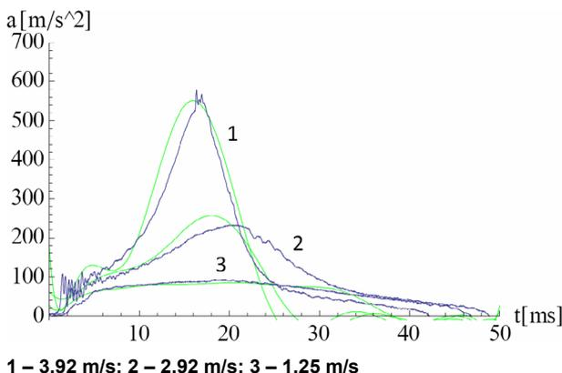
Figure 16. Numerical calculation results (green, lighter lines) and impact tests results (blue, darker lines) for three different impact velocities, specimen 9
