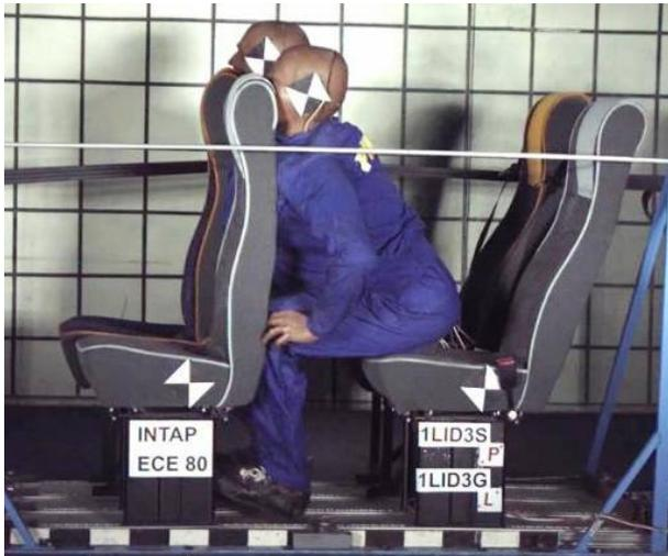
Figure 2. Impact of a head to a head restraint during bus crash test
