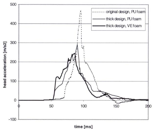
**Figure 1. Head deceleration for three different foam materials [1]**
