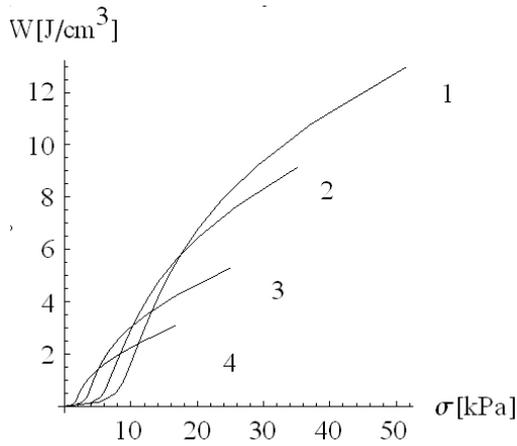
Figure 7. Energy absorption diagram for compression – different specimens and various components proportions
