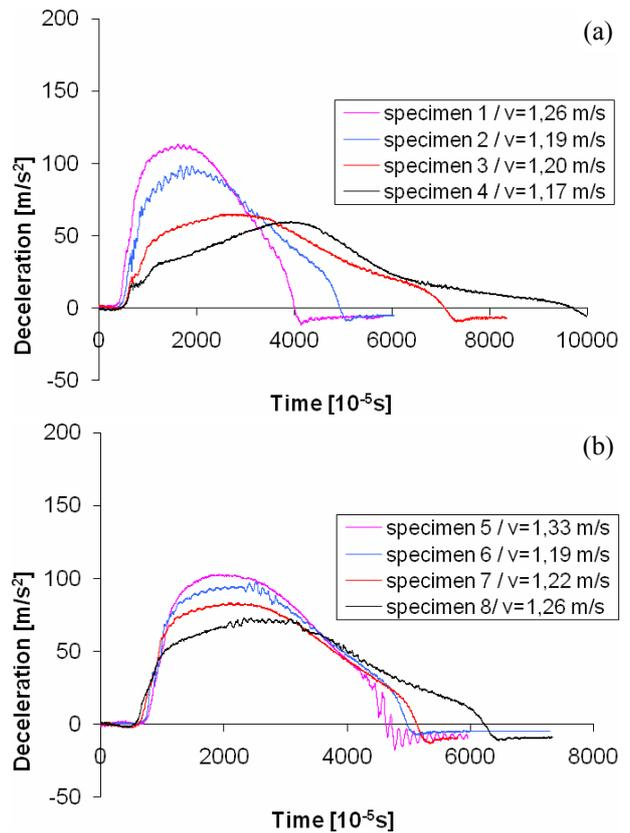
Figure 13. Deceleration vs time for impact velocities about 1.2 m/s: (a) results for specimens of the same densities and various components proportions and (b) results for specimens of the same components proportions and different densities
