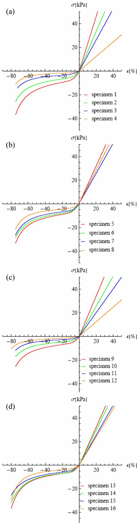
Figure 4. Cumulative diagrams of tension and compression tests results for all specimens: (a) raw material type 2, different components proportions, (b) raw material 2, different densities, (c) raw material 1, different components proportions and (d) raw material 1, different densities
