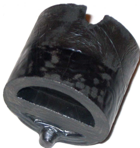
Figure 3. Element of the sunflower huller made of cast basalt
