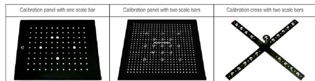
Figure 8. Calibration panels and cross [13]
