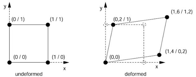
Figure 2. Example for the deformation of a unit square
