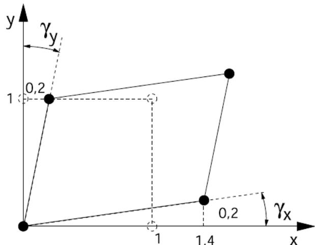
Figure 3. Shear angle definition
