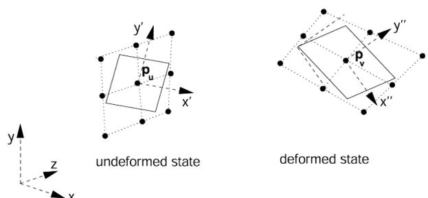
**Figure 6. Definition of the local surface strain coordinate system in 3D**
