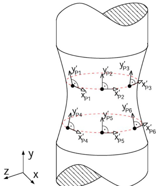
**Figure 5. Definition of the undeformed local surface strain coordinate system in 3D**
