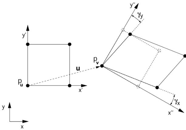
**Figure 4: Definition of the coordinate systems (based on the deformation of a unit square)**
