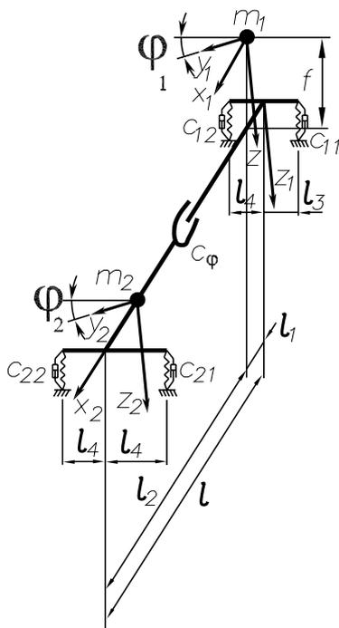
Figure 3. Mechanical model of MLRS vehicle reinforced frame
