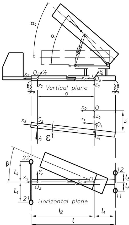
Figure 2. MLRS mechanical model
