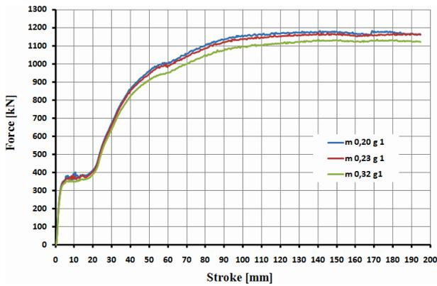
**Figure 10. Force versus stroke diagram – dynamic numerical simulations for  $\gamma = \text{const}$ .**
