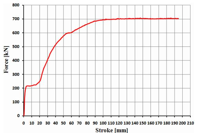
Figure 8. Force versus stroke diagram – quasi-static numerical simulations
