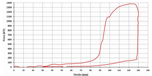
**Figure 15. Force versus stroke diagram – absorption couple S1-P8 –  $V = 19.7$  km/h**
