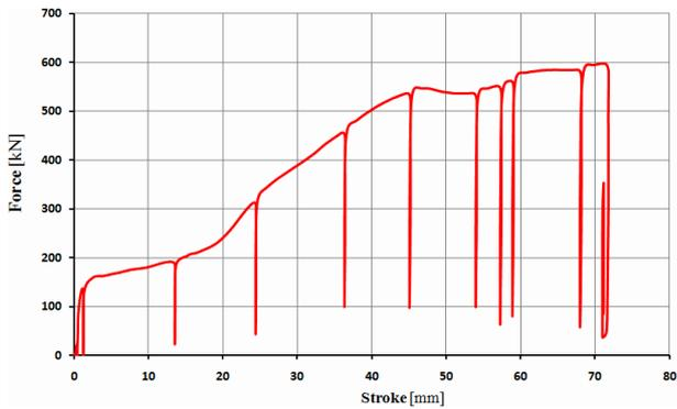
**Figure 11. Force versus stroke diagram – absorption couple S1-P8 – quasi-static test**
