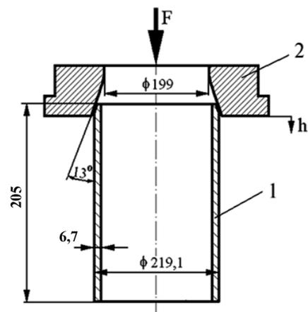
Figure 1. Principle of the functioning of tube absorber
