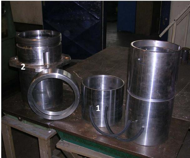
Figure 4. Elements of tube shrinking absorber type samples
