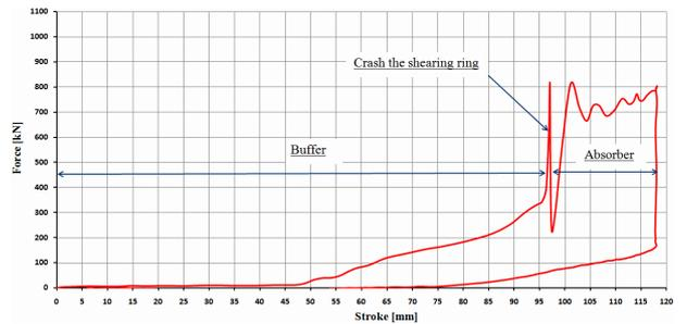
**Figure 14. Force versus stroke diagram – absorption couple S2-P9 –  $V = 11.4$  km/h**
