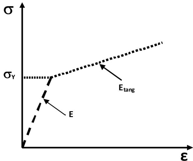
Figure 3. Bilinear characteristic of material
