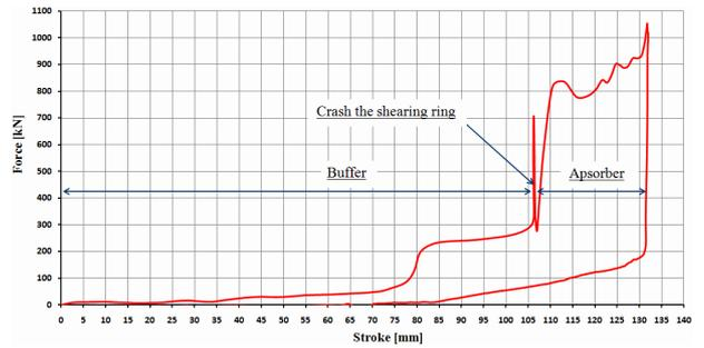
**Figure 13. Force versus stroke diagram – absorption couple S1-P8 –  $V = 11.4$  km/h**
