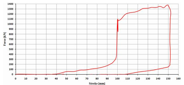
**Figure 16. Force versus stroke diagram – absorption couple S2-P9 –  $V = 19.7$  km/h**
