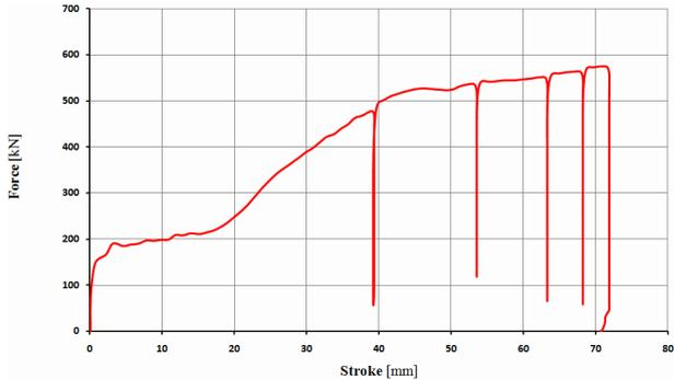
**Figure 12. Force versus stroke diagram – absorption couple S2-P9 – quasi-static test**
