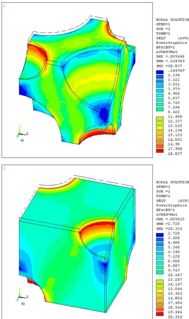
**Figure 3.** Von Mises stress distribution (stress values are in  $\text{daN/mm}^2 = 10^1 \text{ MPa}$ ): (a) in the porous composite, for the two-phase unit cell model with the composite that contains 0.262  $V_f$  and 0.0565  $V_p$ ; (b) in the PLLA matrix, for the three-phase unit cell model with 0.262  $V_f$  and 0.0565  $V_p$ .
