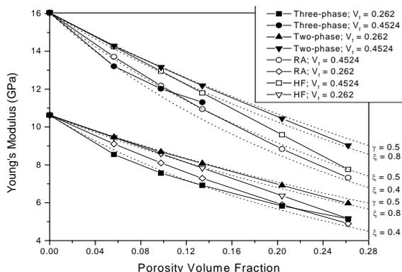
**Figure 4. Young's modulus versus porosity for FE calculations and theoretical models. HT and modified HS predictions are represented by dotted lines .**
