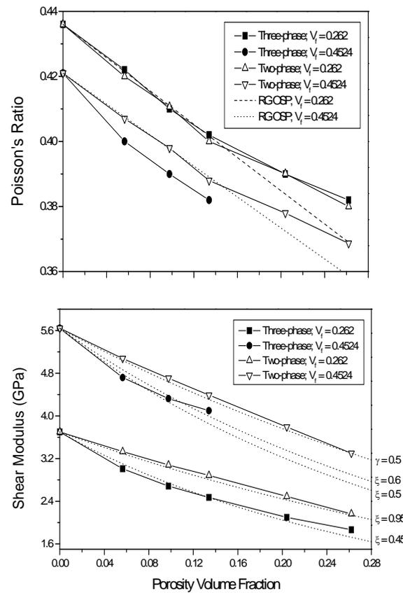
**Figure 5. Poisson's ratio and shear modulus versus porosity for FE calculations and theoretical models. HT**
