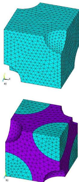
**Figure 2. FE grid of unit cell model with 0.262 particle volume fraction ( $V_f$ ) and 0.0565 porosity volume fraction ( $V_p$ ): (a) two-phase model; (b) three-phase model.**
