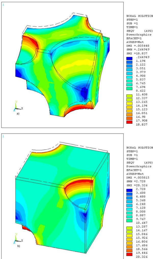
**Figure 3.** Von Mises stress distribution (stress values are in  $\text{daN/mm}^2 = 10^1 \text{ MPa}$ ): (a) in the porous composite, for the two-phase unit cell model with the composite that contains 0.262  $V_f$  and 0.0565  $V_p$ ; (b) in the PLLA matrix, for the three-phase unit cell model with 0.262  $V_f$  and 0.0565  $V_p$ .
