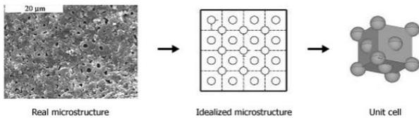
**Figure 1. Idealization of the random pore distribution, shape and size by arranging the pores on a FCC packing array**
