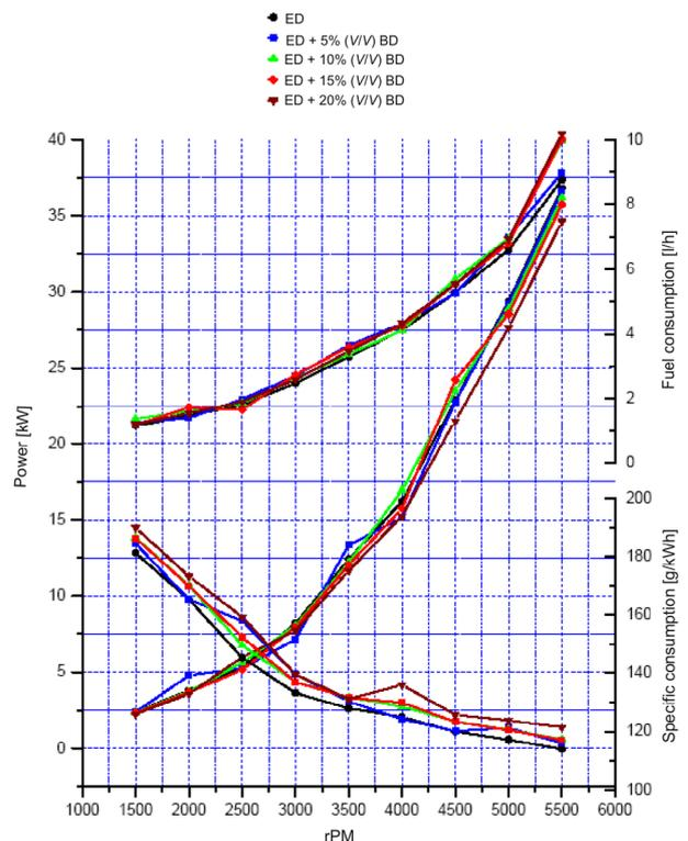
Figure 7: Comparative engine flat road load characteristics recorded for operation with ED and blends of ED and BD
