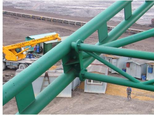
**Figure 5. Part of a superstructure of a wheel excavator made of pipes**
