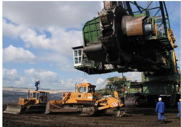
**Figure 22. Attaching a bulldozer to the bucket wheel boom**
