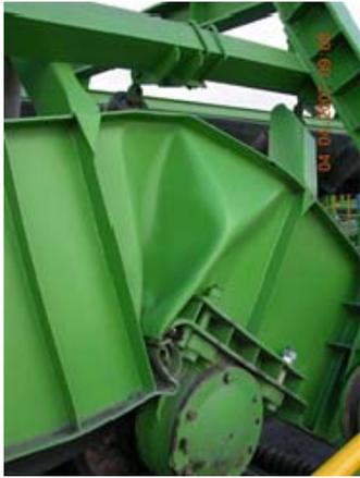
**Figure 8. Frame of the conveyor belt with damaged superstructure**
