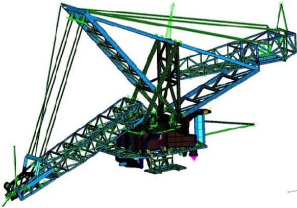
Figure 14. Model of excavator with a portal
