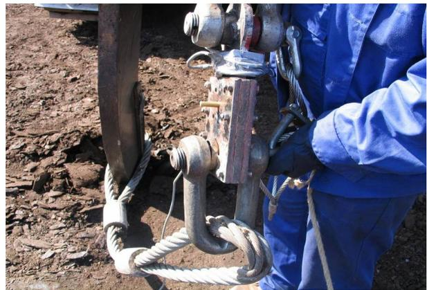
**Figure 21 Device used to quickly release the mass after reaching the given force**
