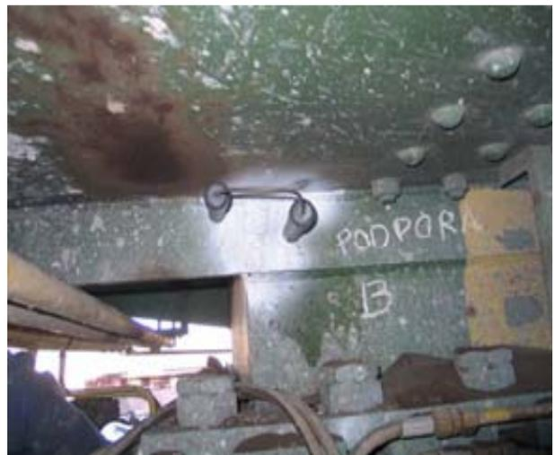
**Figure 25. Nondestructive test of an excavator joint**
