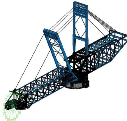
**Figure 12. Hoisting system of the SChRs 4600.50 excavator**
