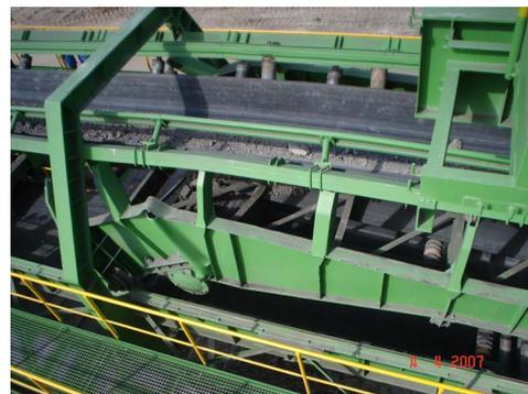
**Figure 7. Loss of local stability of the supporting beam in the frame of a conveyor belt**
