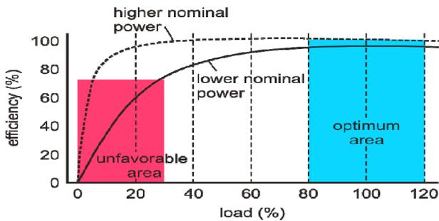
Figure 13. Efficiency of asynchronous motors [4]
