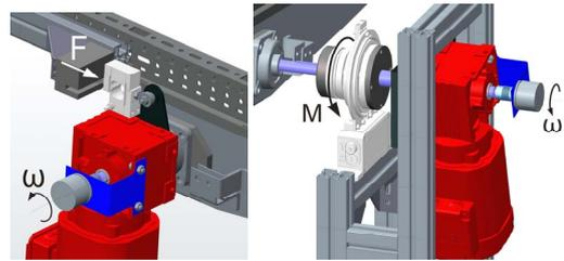
Figure 7. Measurement setups for mechanical power
