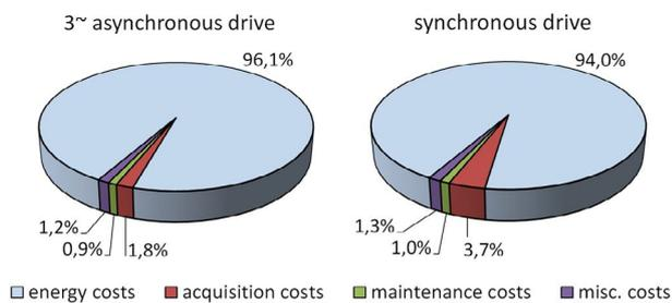
Figure 14. Life cycle costs for different motor types [5]
