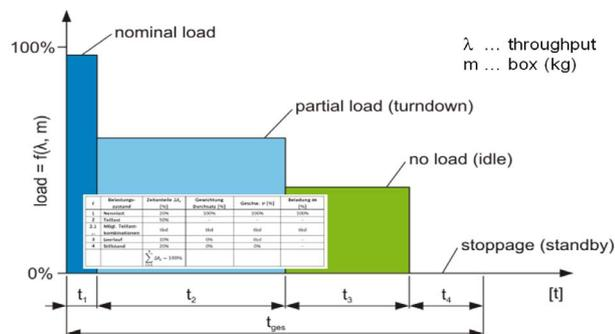
Figure 16. Example - representative operation cycle (ROC)
