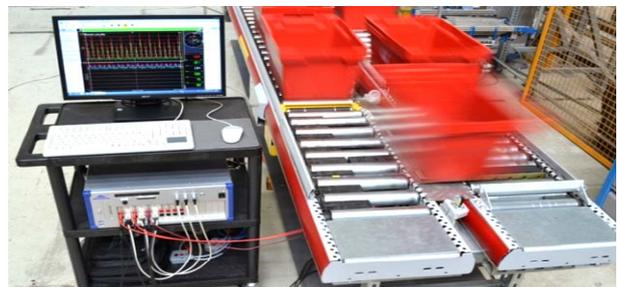
Figure 4. Roller conveyor – flat belt operated (RC-FB)
