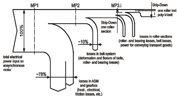
**Figure 12. Power losses of RC-FB (load 25kg)**
