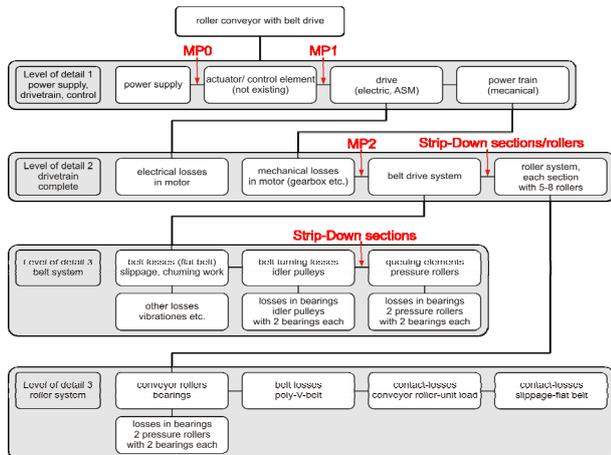
Figure 6. Schematic buildup and measuring points (RC-FB)
