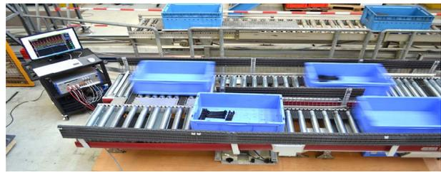
Figure 3. Roller conveyor - drum motors (RC-DM)
