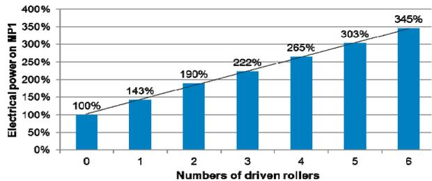
**Figure 10. Power consumption of roller elements**
