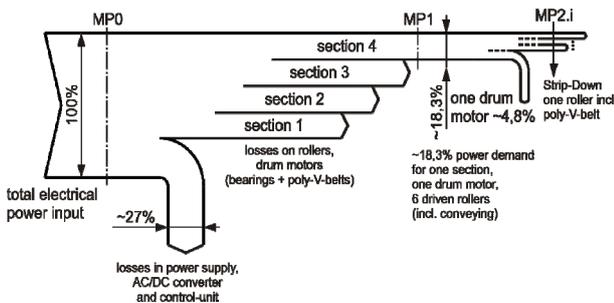
**Figure 9. Power losses of RC-DM (load 25kg)**
