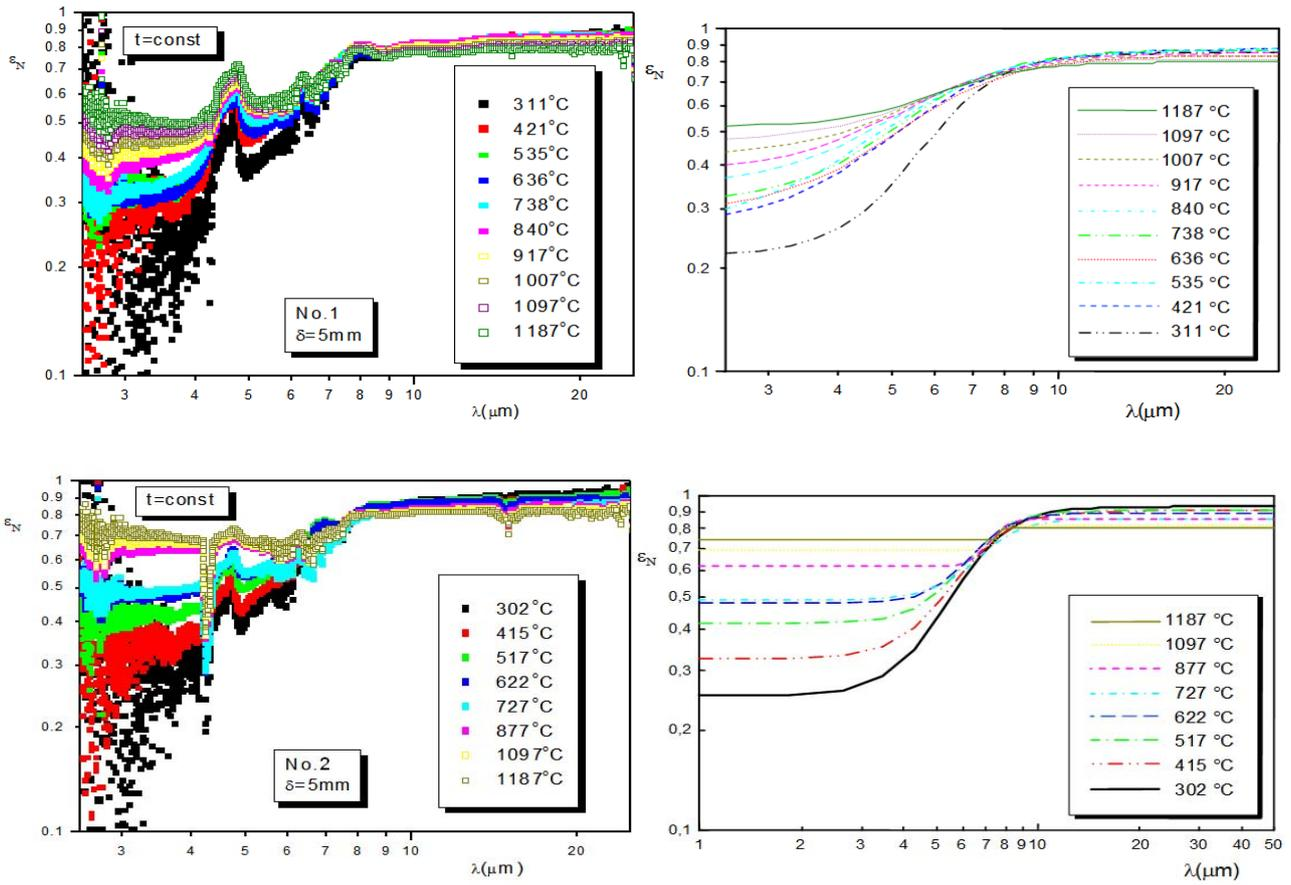
Figure 5. Spectra of ash deposit emittance in heating mode (left=experiment; right=fit)
