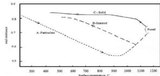
Figure 1. Ash total emittance vs. temperature [1]
