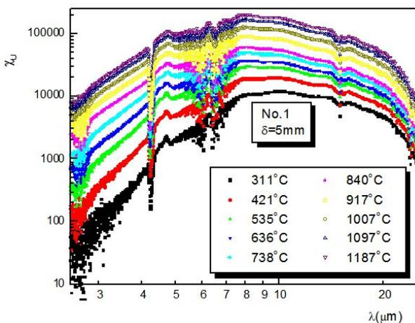
Figure 4. IR emissive power spectra of ash - heating
