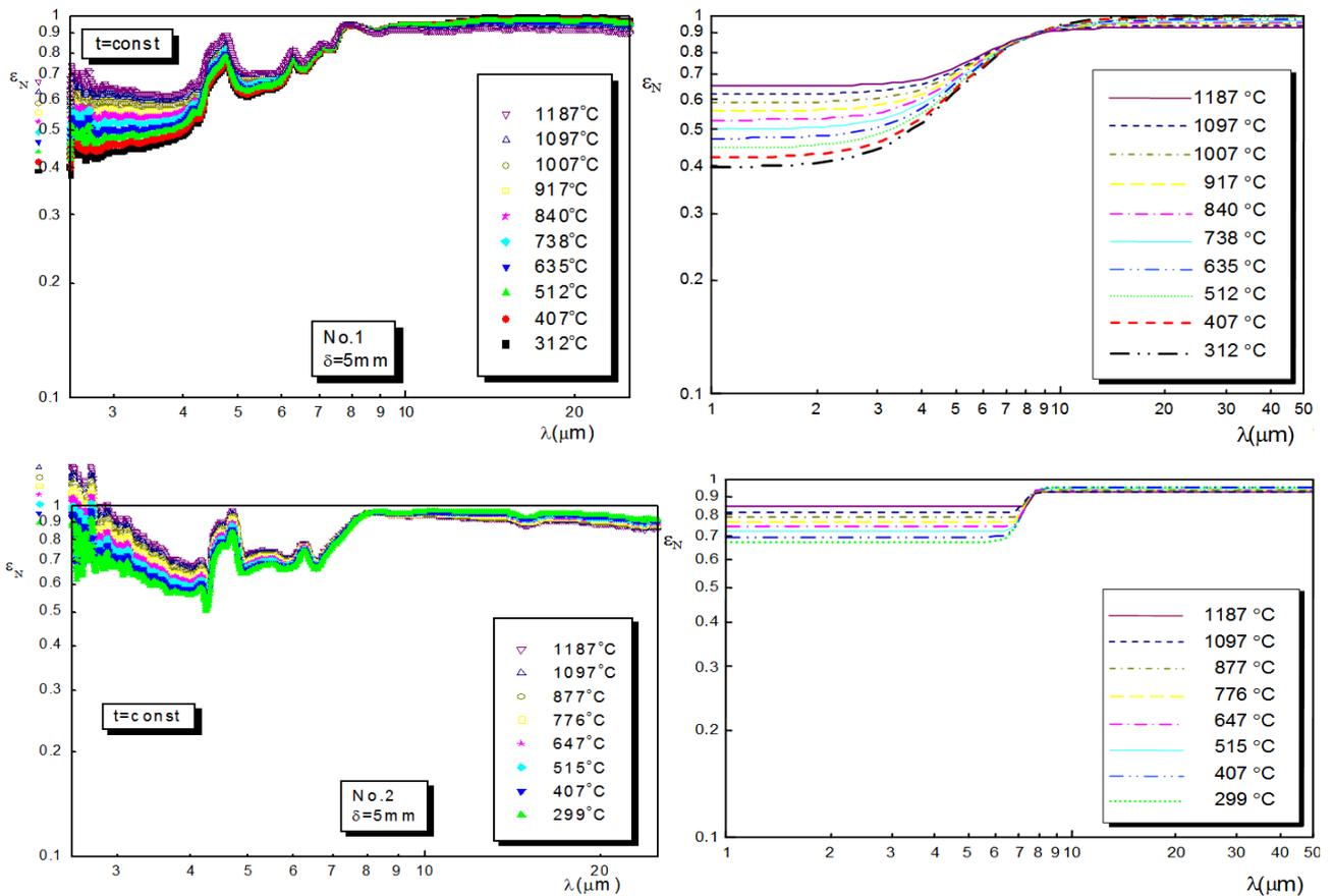
Figure 6. Spectra of ash deposit emittance in cooling mode (left=experiment; right=fit)
