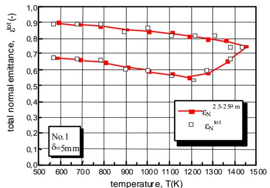
Figure 3. Total emittance vs. temperature of ash
