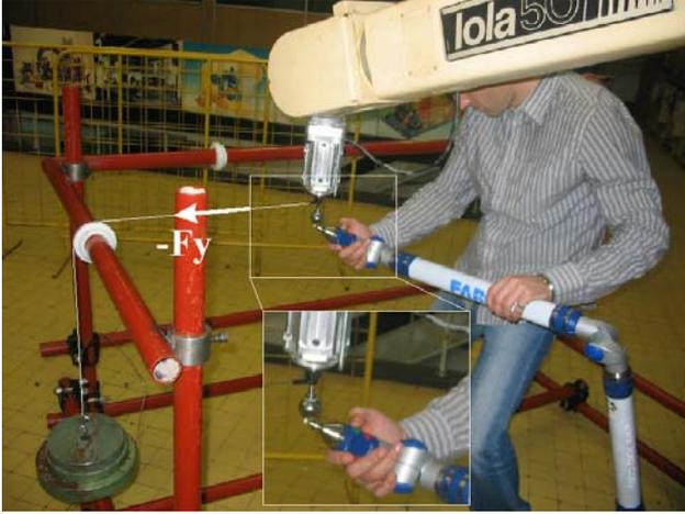
Figure 10. Experimental setup of robot loading and displacements measurement
