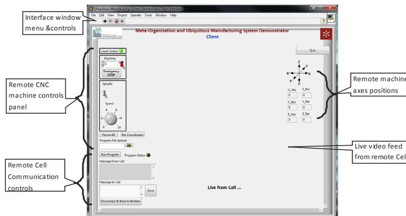
Figure 2. Functional Presentation of Remote Control User Interface
