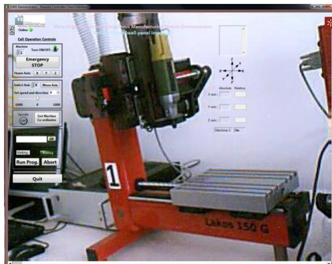
Figure 4. "Wall Interface" of Remote Client for Operations on Cell
