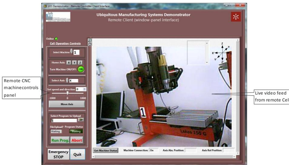
Figure 3. "Window Interface" of Remote Client for Operations on Cell
