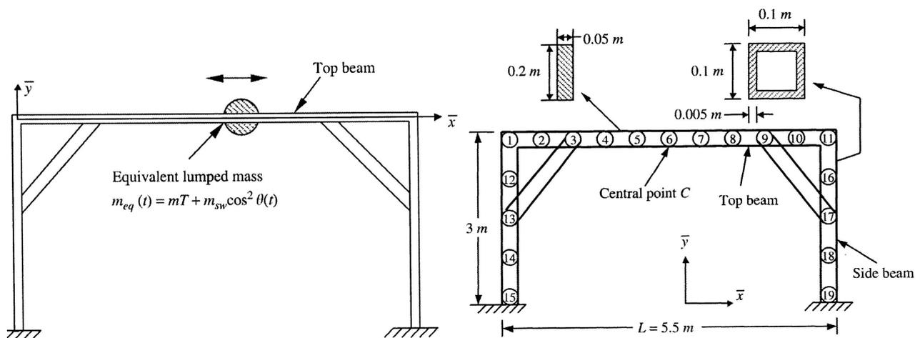
Figure 4. Wu's mathematical model for a crane hoisting a swinging mass [8]
