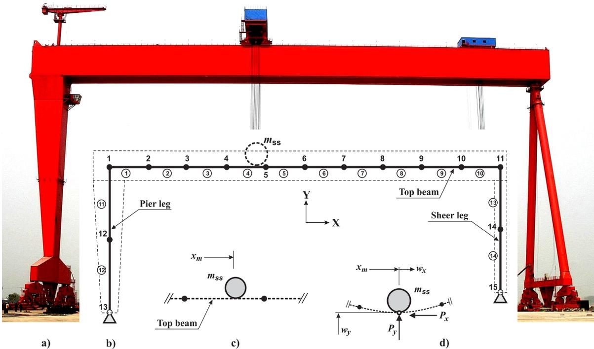
Figure 9. a) Real model of the gantry crane, b) FE model of the framework, c) Moving mass, d) Dynamic interaction [16]
