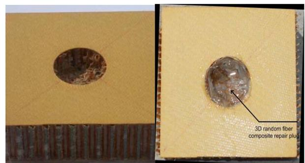
**Fig. 4. a) Prepared panel for plug insertion, b) 3D random fiber composite core plug**
