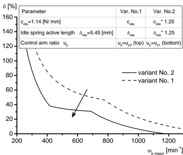
Figure 5. Comparison of two different governor's setups; goal: lowering the  $\delta$  over entire engine speed range
