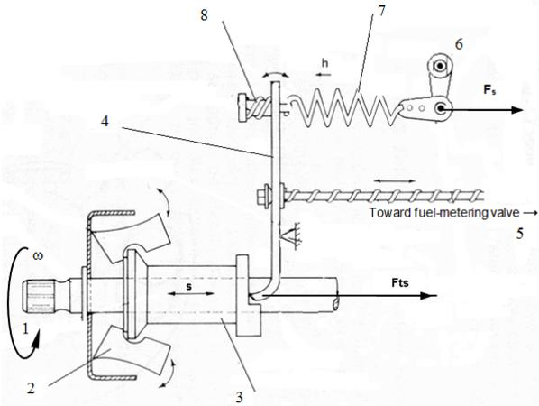
**Figure 1. The variable speed governor of DPA type rotary pump - main variables of the governor's mathematical model.**
