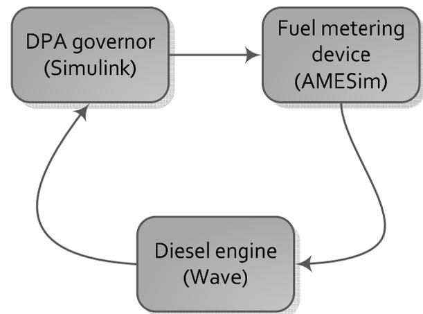
Figure 6. Multiple model co-simulation concept for testing a complex multi-domain physical systems.
