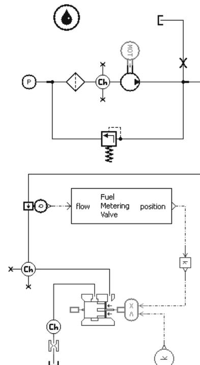
Figure 7. Schematics of the Diesel engine submodel in WAVE™ (left) and fuel metering device in AMESim™ (right)
