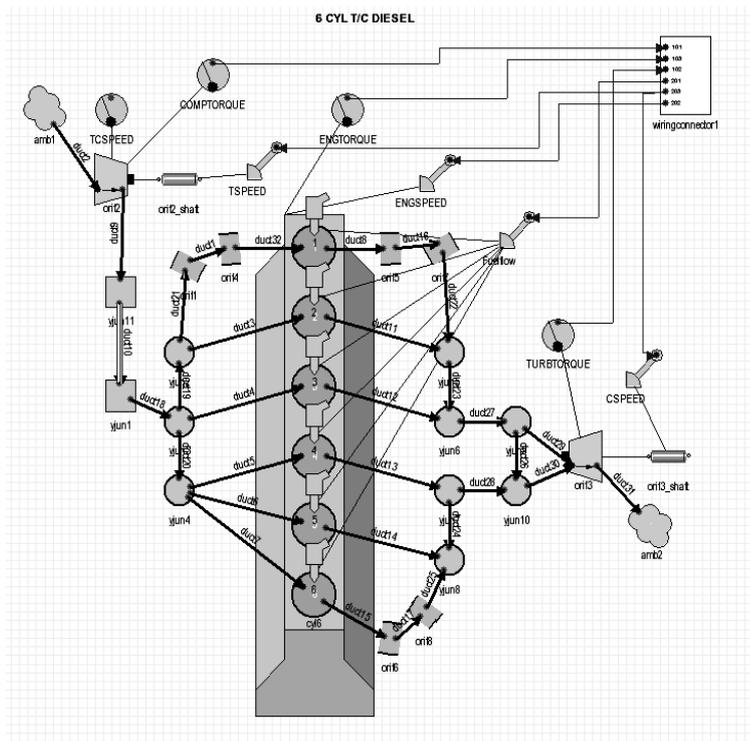
The overall capabilities of the WAVE™ simulation software provided a realistic simulation of a general turbo charged diesel engine processes – since the specific engine data are irrelevant for this type of testing. The schematic of the WAVE™ engine model is shown in Figure 7 (left).
