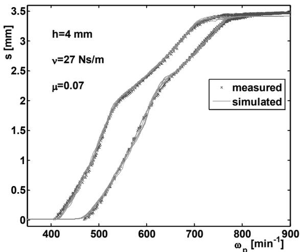
Figure 3. Measured and simulated characteristic of the governor – a comparison.
