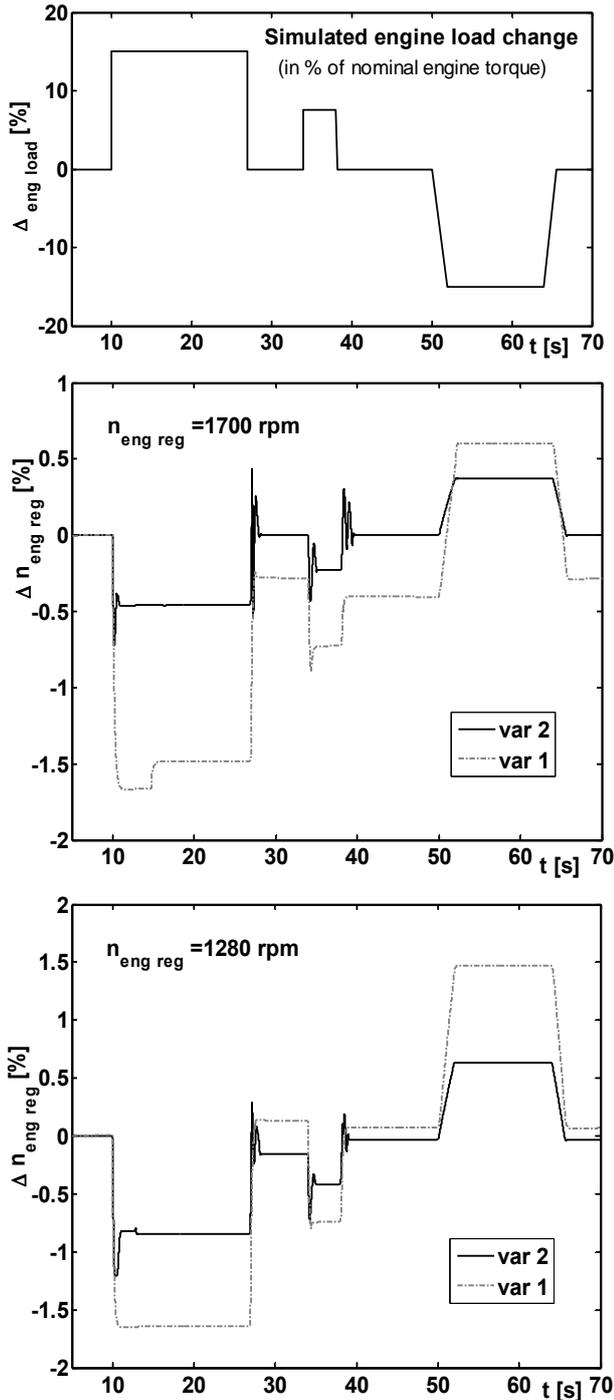
Figure 8. Comparison of two different governor's setups (refer to Fig. 5); Governed engine speed – 1700 rpm (middle) i.e. 1280 rpm (bottom); Engine load torque variation sequence (top).
