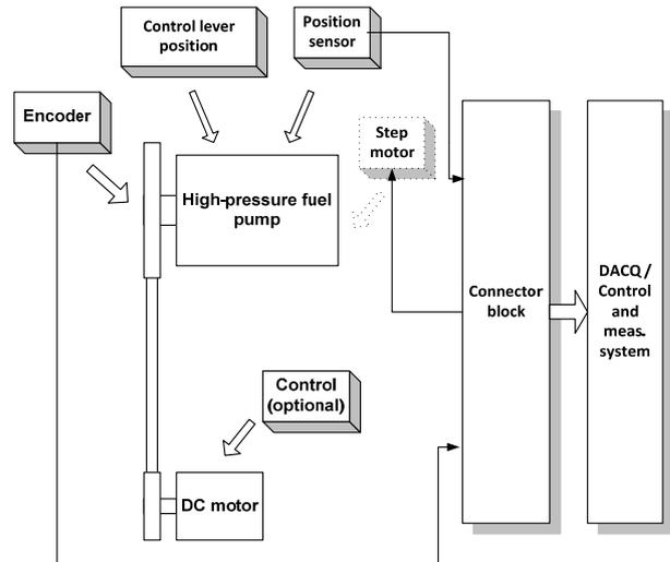
Figure 2. Schematic of the test bench installation for the dynamical testing of the speed governor
