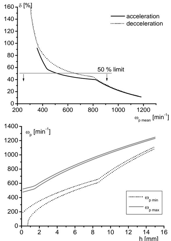
Figure 4. Driveshaft speed limits (bottom); Inequality factor  $\delta$  (top); Hysteresis as an effect of friction losses.
