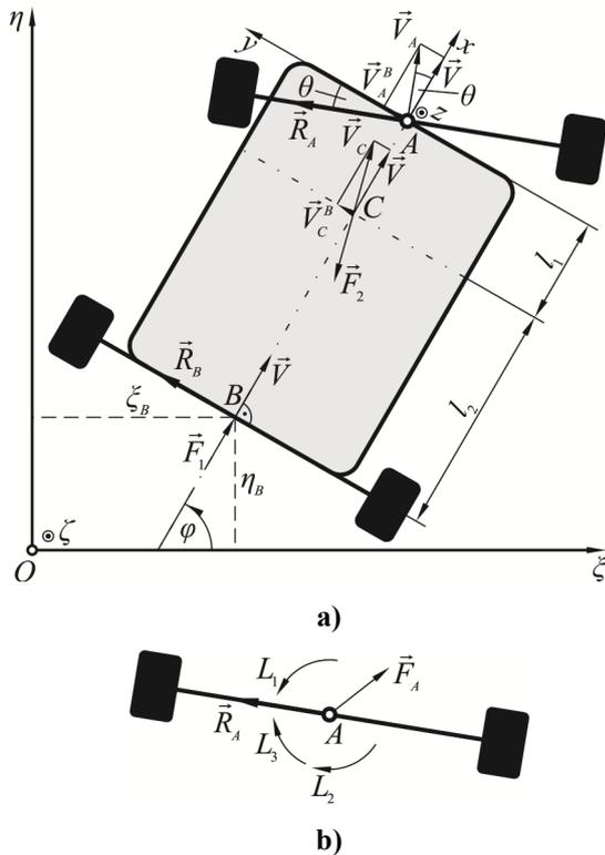
Figure 1. a) Simplified vehicle model; b) front axle.
