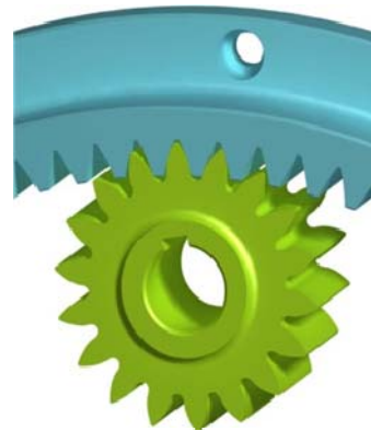
Figure 2. Internal gearing with HCR profile of teeth flanks
