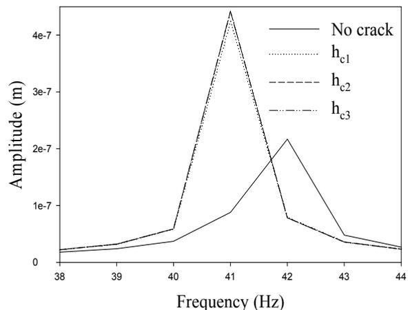
Figure 8. FRF for crack position  $l_{c3}$  for different crack depth at third natural frequency
