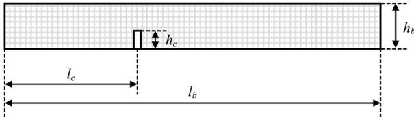
Figure 1. Beam model with single transversal crack
