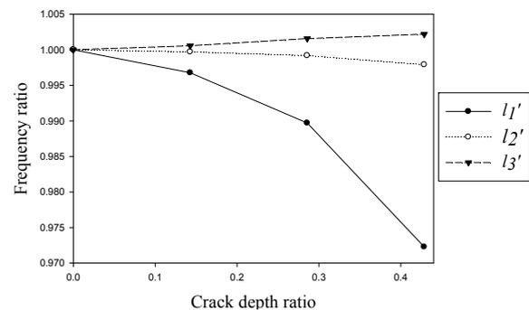
Figure 2. First natural frequency ratio  $\omega_1'$  in terms of crack depth ratio for different crack positions
