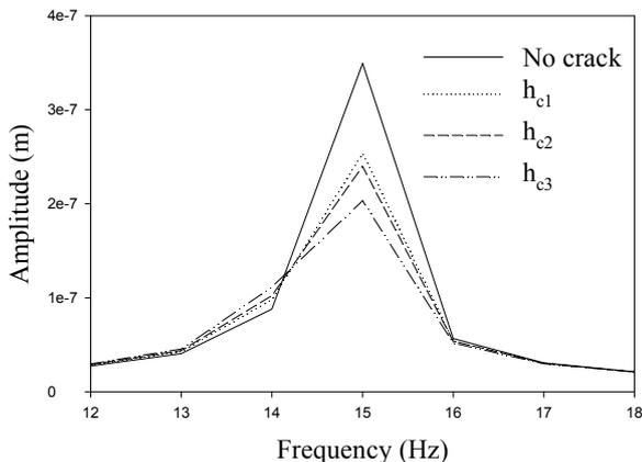
Figure 5. FRF for crack position  $l_{c2}$  for different crack depth at second natural frequency
