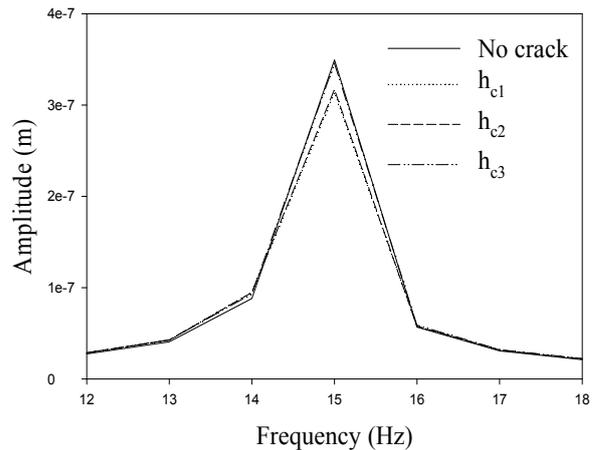
Figure 6. FRF for crack position  $l_{c3}$  for different crack depth at second natural frequency
