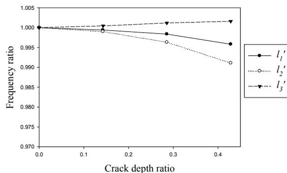
Figure 4. Third natural frequency ratio  $\omega_3'$  in terms of crack depth ratio for different crack positions
