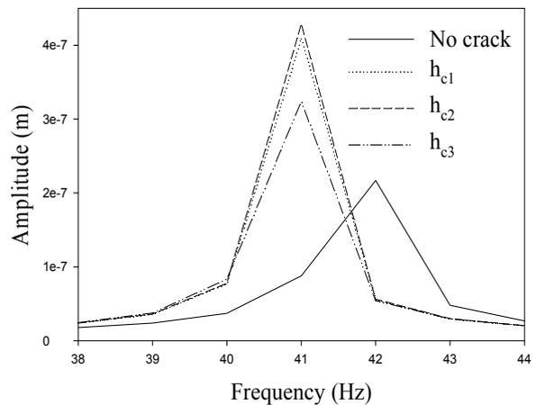
Figure 7. FRF for crack position  $l_{c2}$  for different crack depth at third natural frequency
