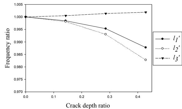
Figure 3. Second natural frequency ratio  $\omega_2'$  in terms of crack depth ratio for different crack positions
