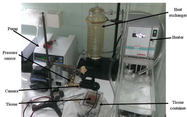
Figure 4 - Architecture of the system designed for the experiment
