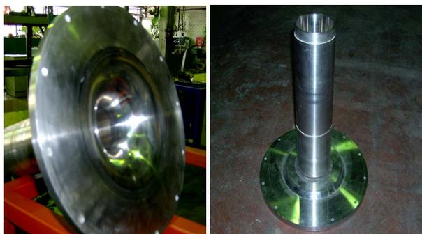
Figure 8. Two photos of a manufactured CFV: front view at the entrance to the nozzle (left), and side view at the Venturi nozzle (right) [9]
