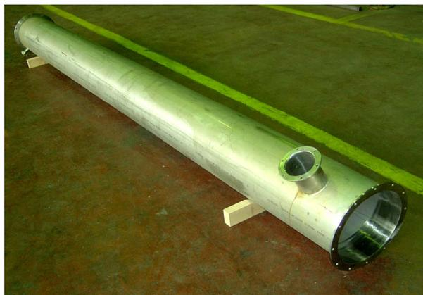
**Figure 3. Front view of the dilution tunnel with the flange for the exhaust pipe**
