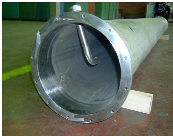
**Figure 4. Rear view of the dilution tunnel with isokinetic sampling probe**
