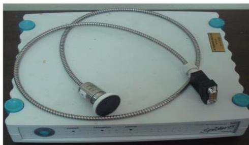
Figure 4. Sensor and A/D converter
