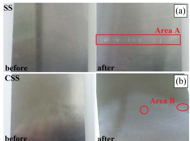
Figure 6. Block species before and after the tests: (a) stainless steel (SS) and (b) chromium coated stainless steel (CSS)
