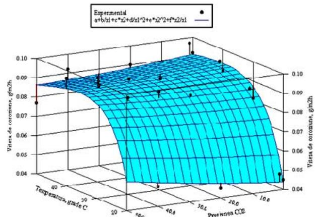
Figure 5. Corrosion rate vs. temperature and CO<sub>2</sub> pressure for carbide sprayed piston in couple with hard chromium cylinder in active anode Al-Zn presence
