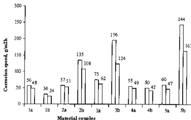
**Figure 1. Corrosion rate at 20 °C and CO<sub>2</sub> barbotage;**
