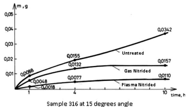
Figure 15. Erosion wear curves at impingement angle of 15°
