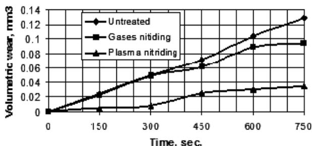
Figure 14. Wear curves for AISI 316 samples
