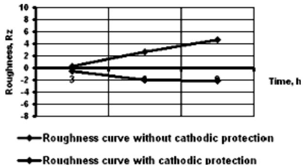
**Figure 11. Roughness modification curve for surface of material GJL-HB215 at 15° impingement angles**
