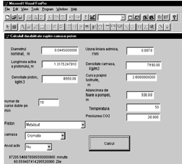
Figure 9. Program simulation for sucker rod pumps durability calculus
