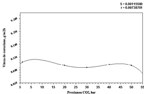
Figure 3. Corrosion rate vs. CO<sub>2</sub> pressure for carbide sprayed piston in couple with hard chromium cylinder
