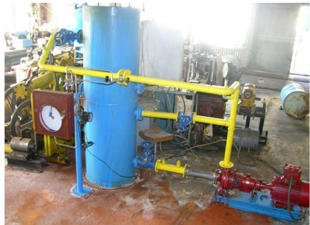
**Figure 12. Centrifugal pumps testing stand**
