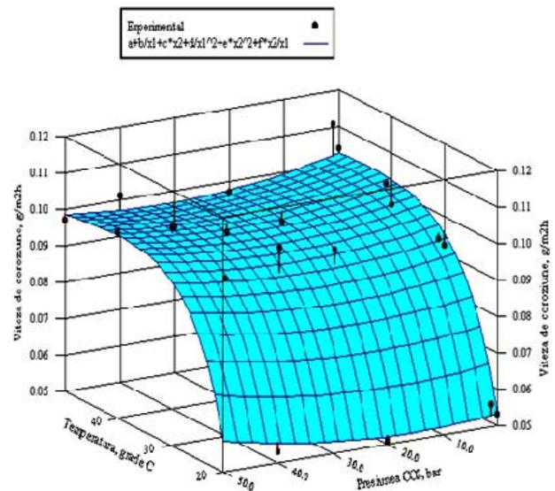
Figure 4. Corrosion rate vs. temperature and CO<sub>2</sub> pressure for carbide sprayed piston in couple with hard chromium cylinder
