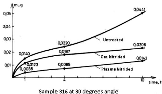
Figure 16. Erosion wear curves at impingement angle of 30°
