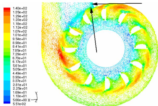
Fig. 5. Velocity vectors of the mixture on the exit from the ventilation mill, in place near suction plates and on the start of duct
