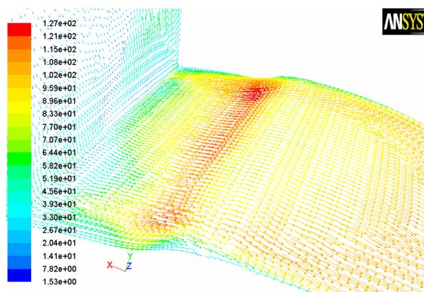
**Fig. 7. Absolute velocity vectors of the particles of sands near the walls and area of suction plates of mill**
