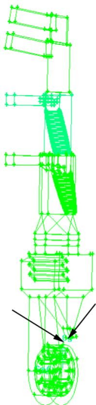
Figure 3. The geometric model of the ventilation mill with duct and channels to the entrance at the burner
