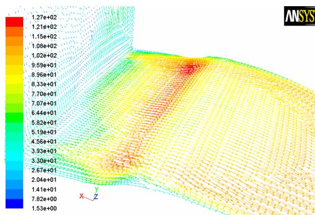
**Fig. 7. Absolute velocity vectors of the particles of sands near the walls and area of suction plates of mill**
