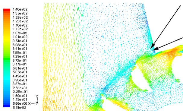
Fig. 6. Detail velocity vectors of the mixture on the exit from the ventilation mill, in place near suction plates and on the start of duct (area of suction plates is shown by arrows)
