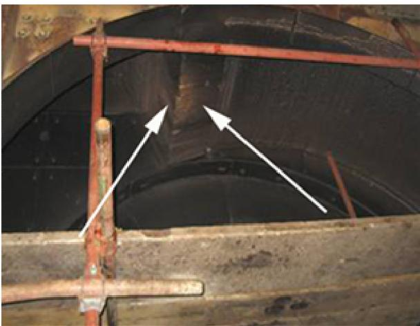
Figure 2. Position of suction plates in the working well of ventilation mill
