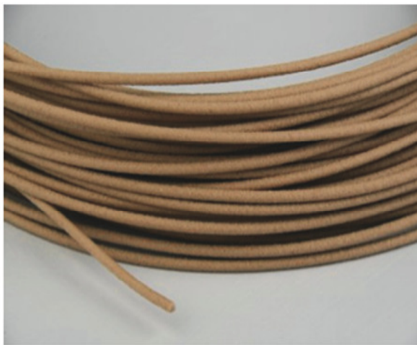
Figure 4: Plastic with 40% recycled wood [www.lulzbot.com]
