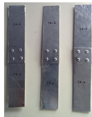
Figure 4. Riveted specimens for tensile testing
