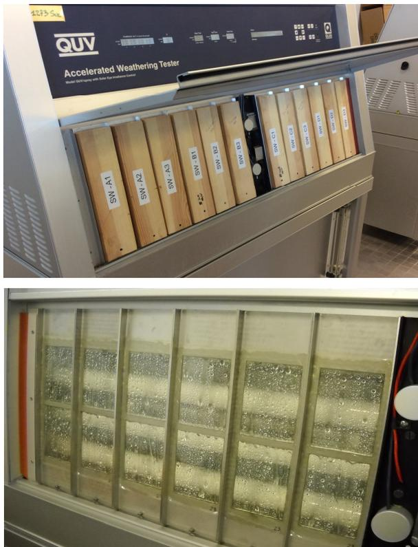
**Figure 1. Coated wood panels (left) and free coating films (right) exposed to artificial weathering**
