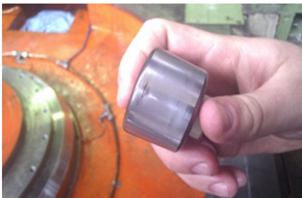
Figure 3. Mechanical damage of rolling bearing
