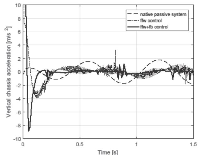
Figure 12. Vertical chassis acceleration comparison
