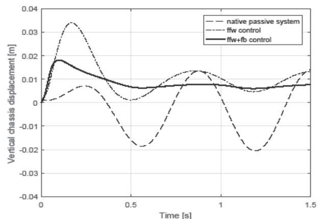
Figure 11. Vertical Chassis Displacement Comparison
