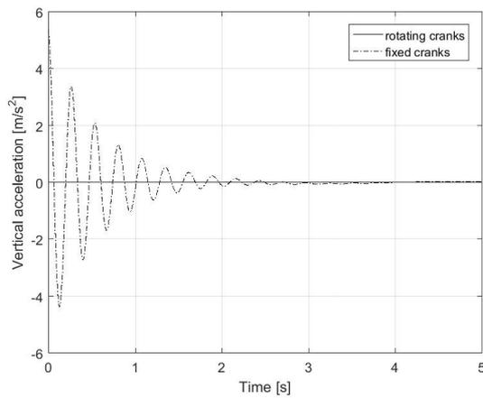
Figure 8. Vertical acceleration for the 1DOF system
