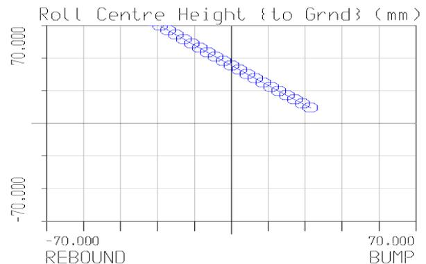
Figure 3. Roll center height to ground variation in bump and rebound for passive system
