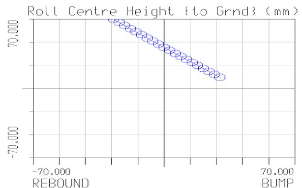
**Figure 3. Roll center height to ground variation in bump and rebound for passive system**
