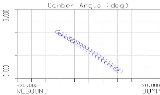
Figure 4. Camber angle variation in bump and rebound for passive system
