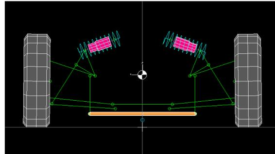
**Figure 2. Kinematic simulation implemented in LSA**
