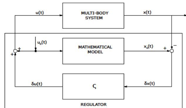
Figure 10. Closed loop control scheme
