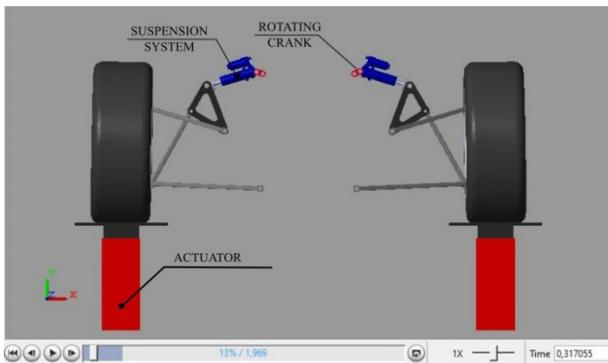
Figure 9. Multi-body half model of the race car
