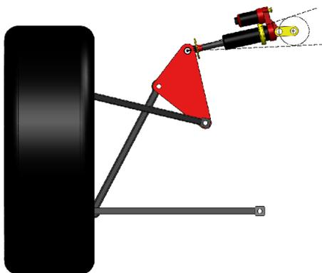
**Figure 1. Original system retrofitted with new mechanical link to chassis**
