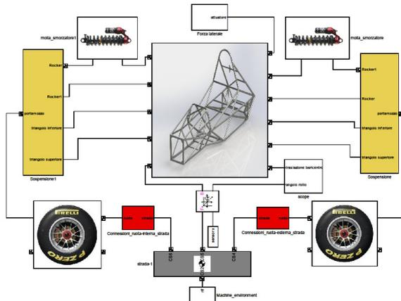
Figure 5. Multi-body model of system, Simulink interface
