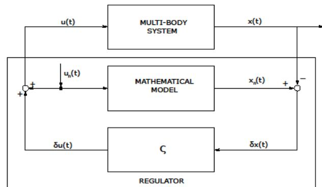
Figure 10. Closed loop control scheme
