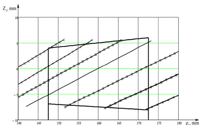
Figure 5. Lines of action on the pinion tooth surface
