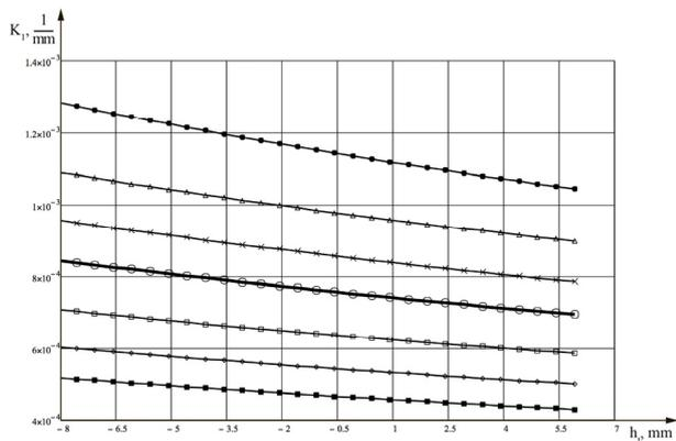
**Figure 6. Results of calculation of the principal reduced curvature in meshing**
