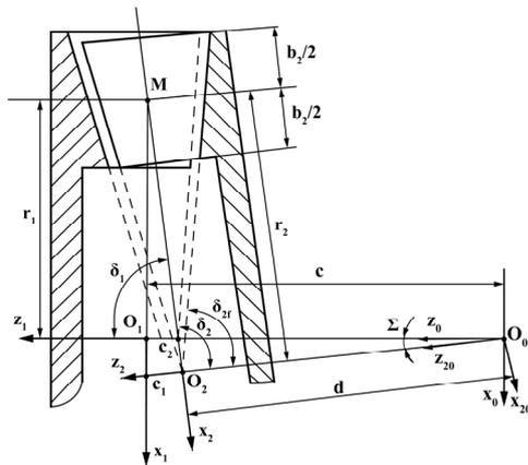
**Figure 4. Design scheme of the straight bevel gears with a small shaft angle with a non-generated gear and a generated pinion and a scheme of coordinate transformation from the coordinate system S2 to the coordinate system S1**
