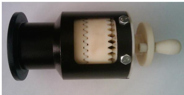
**Figure 7. Model of the coaxial gearbox with a precessional bevel gear with a small shaft angle**
