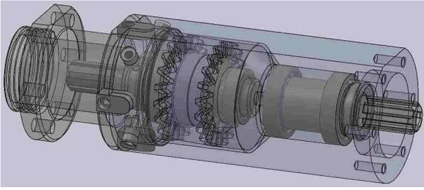
**Figure 1. Coaxial gearbox based on a bevel gears with a small shaft angle**
