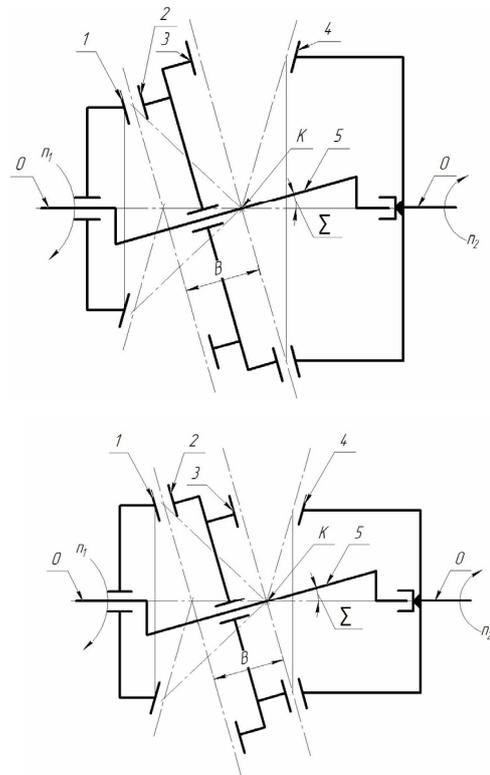
**Figure 3. Coaxial gearbox scheme, gear coupling module is larger (a) or smaller (b) than bevel precessional gear**
