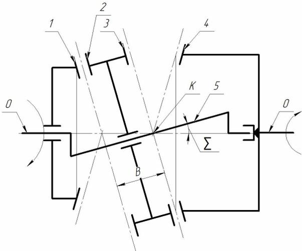
**Figure 2. Scheme of coaxial gearbox based on precessional bevel gear**
