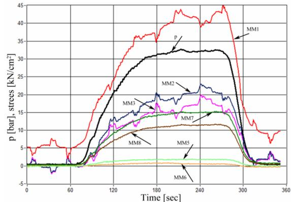
Figure 5. Measured stress as a function of pressure, after material at MM1 was plastically deformed (33 bar load, new plastic deformation occurs at MM1)
