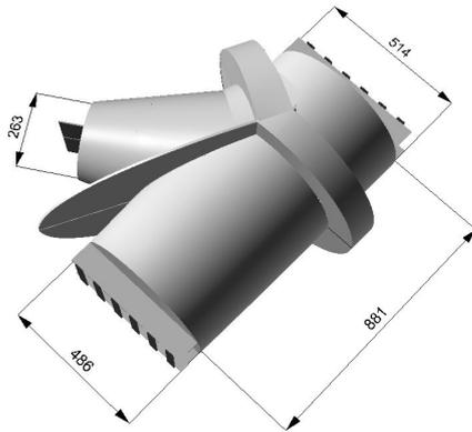
Figure 7. Geometry of the pipe branch model
