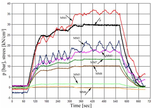
Figure 3. Measured stress as a function of pressure, for pressure value of 30 bar (plastic deformation occurs at MM1)
