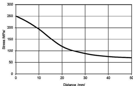
Figure 9. Stress distribution along the surface with distance 50 mm from critical zone at MM1
