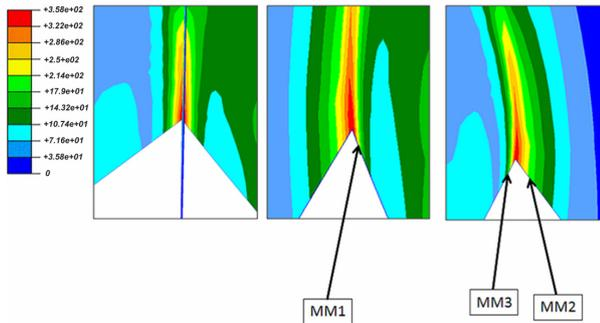
Figure 8. Stresses [MPa] in circumferential (vertical) direction at MM1, MM2 and MM3 measuring locations (p = 20 bar)
