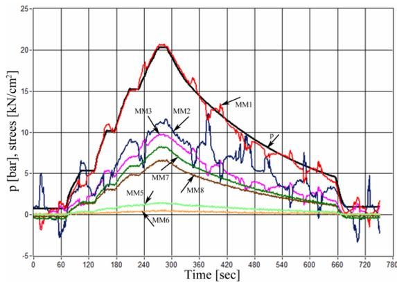
Figure 2. Measured stress as a function of pressure, for pressure values lower than 20 bar
