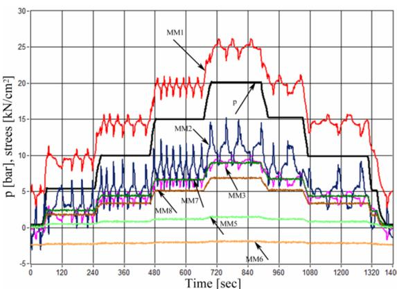
Figure 4. Measured stress as a function of pressure, after material at MM1 was plastically deformed (repeated 20 bar load, new plastic deformation does not occur)
