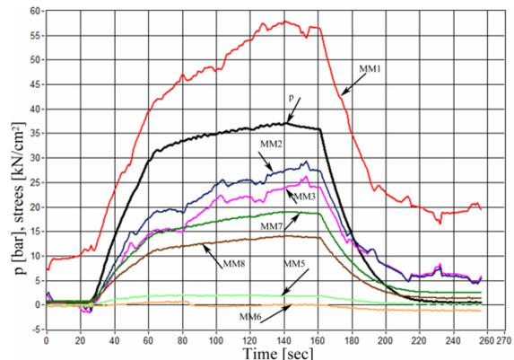
Figure 6. Measured stress as a function of pressure, for pressure value of 37 bar (new plastic deformation occurs at MM1 location and plastic deformation occurs at MM2 location)
