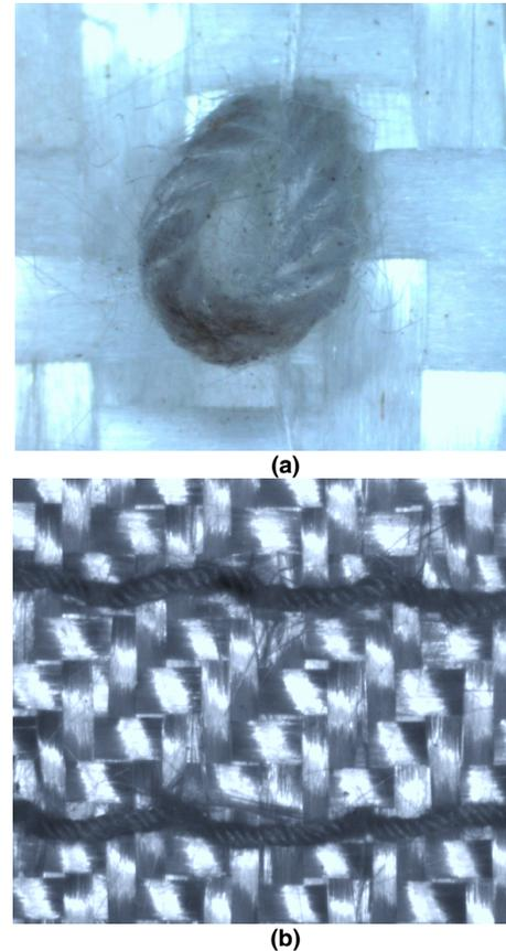
Figure 1. Architectures of tufted preform in front (a) and back face (b).
