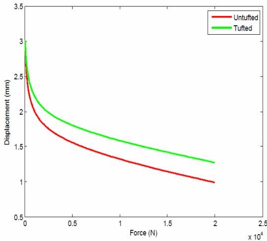
**Figure 8. Load vs. displacement of compression test of preforms.**
