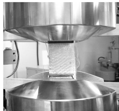
Figure 2. In-plan tensile test setup.
