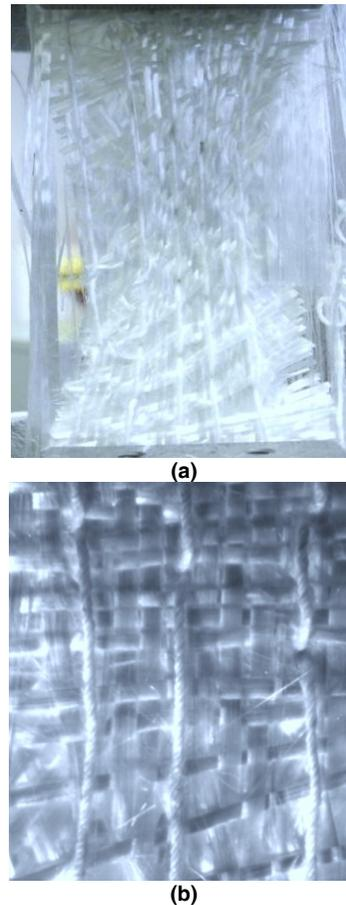
**Figure 9. Tufted preforms subjected to tensile loading a) longitudinal tufted b) transverse tufted.**
