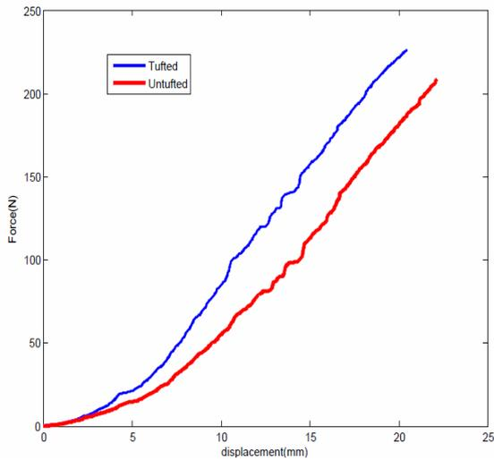
**Figure 7. Load vs. deflection curve of tufted and untufted preforms.**
