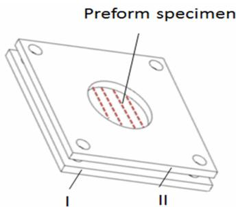
Figure 3. Experimental setup for drapability testing.
