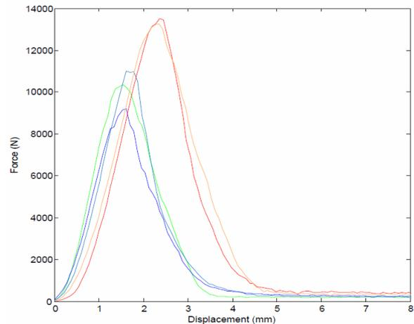
Figure 5. Load Vs Displacement for tufted perform.
