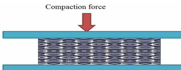
Figure 4. Compression test setup of tufted preform.
