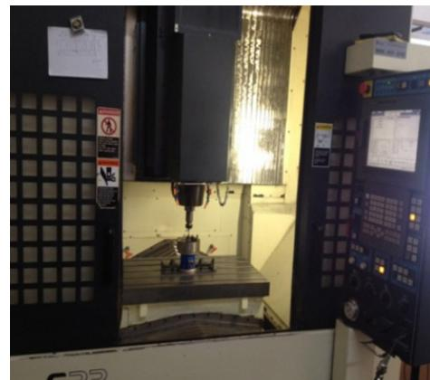
**Figure 4. Vertical CNC machine**
