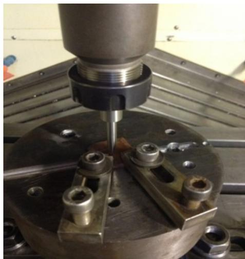
Figure 5. Setup for Drilling
