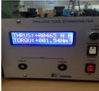
Figure 6. Drill dynamometer
