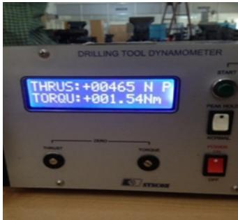
**Figure 6. Drill dynamometer**
