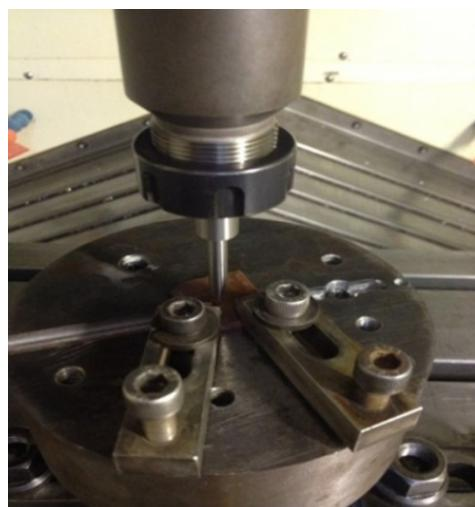
**Figure 5. Setup for Drilling**
