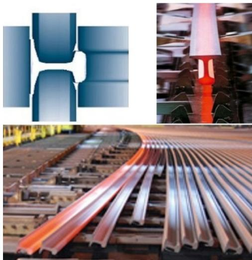
Figure 5. The uneven cooling of rail profile and bending of the rails in cooling bed
