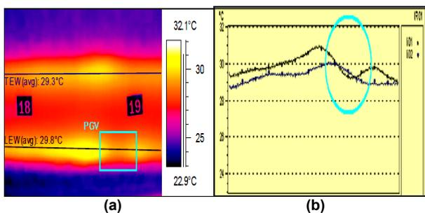
Figure 7. Inspection of adhesive joint showing, (a) Infrared image of glue void and (b) bar graph showing temperature variance along bond line.
