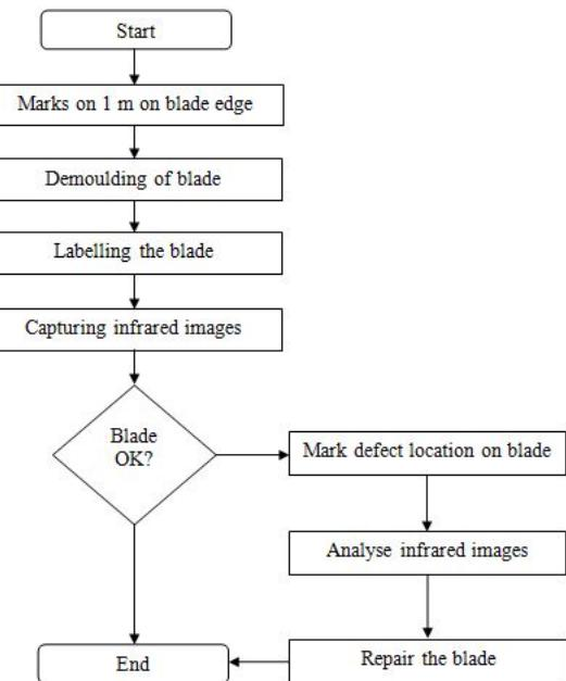
**Figure 2. Flowchart for infrared thermography.**
