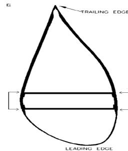
**Figure 1. Main areas of the blade to be inspected**
