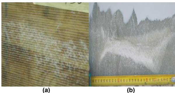
**Figure 10.** Photographs of defects identified by inspection process are (a) dry laminate and (b) wrinkle formation due to fibre disorientation.
