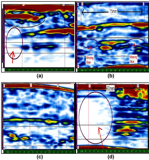
**Figure 9.** Ultrasonic inspection of adhesive joints between main webs and blade shell showing (a) Improper placement of web, (b) narrow bond, (c) wet glue and (d) dry glass
