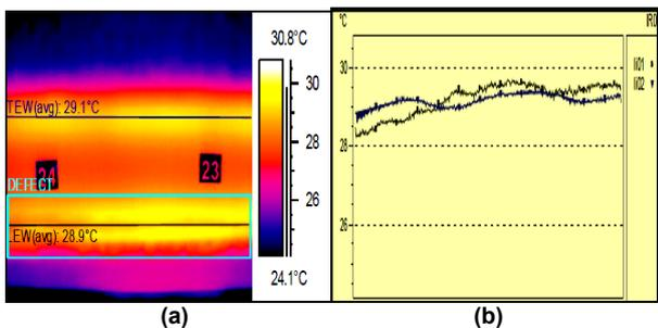
Figure 6. Inspection of adhesive joint showing, (a) Infrared image of dry glass defect and (b) bar graph showing temperature variance.
