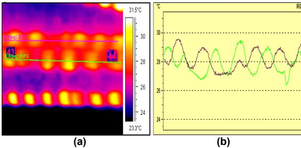
Figure 5. Inspection of adhesive joint showing, (a) Infrared image of spot curing glue defect and (b) bar graph showing temperature variance.
