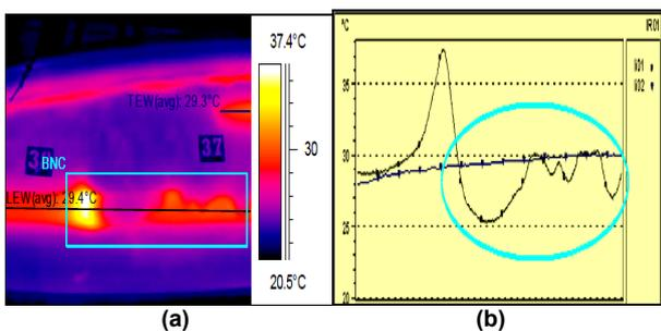
Figure 8. Inspection of adhesive joint showing, (a) Infrared image of uncured bond and (b) bar graph showing temperature variance along bond line.
