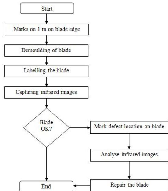
Figure 2. Flowchart for infrared thermography.
