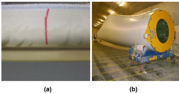
Figure 3. (a) Reference marking at 1 meter interval and (b) Placing the blade with trailing edge upwards.
