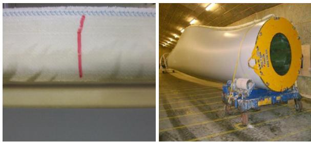
**Figure 3. (a) Reference marking at 1 meter interval and (b) Placing the blade with trailing edge upwards.**
