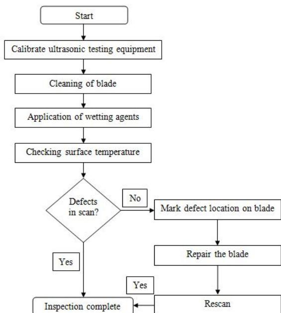
**Figure 4. Flowchart for ultrasonic testing.**
