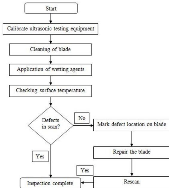
Figure 4. Flowchart for ultrasonic testing.
