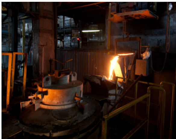
Figure 6. Final phase of the casting process with an active control of the temperature of molten iron.
