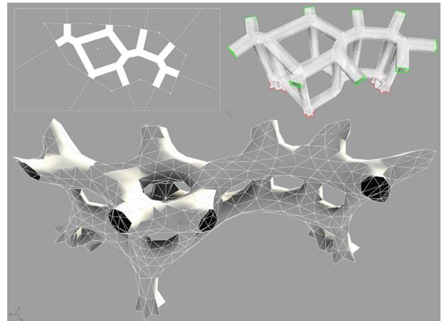
**Figure 3. Initial voronoi points and lines selected (Top left). Top right, shows the two sets of voronoi trusses connected with vertical columns. The green naked edges are anchors with not much strength and the red naked edges of the base have very strong strength. (Bottom), the triangulated mesh obtained after the relaxation method described. (Image by authors).**
