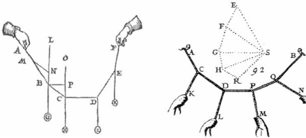
**Figure 2. (Left) One of Stevin's drawings of force equilibrium of hanging weights on a string (1586), and (Right) an illustration by Varignon showing a graphical analysis of a funicular shape (1725). [17]**
