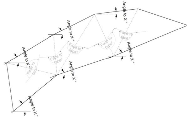
Fig 9. Each stripe is analyzed in the naked cantilever with the X axis, and in the folding angle between faces. The average angles are compared in the graph (fig.10). (Image by author)
