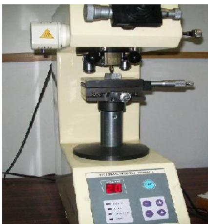
Figure 3 Vickers hardness tester
