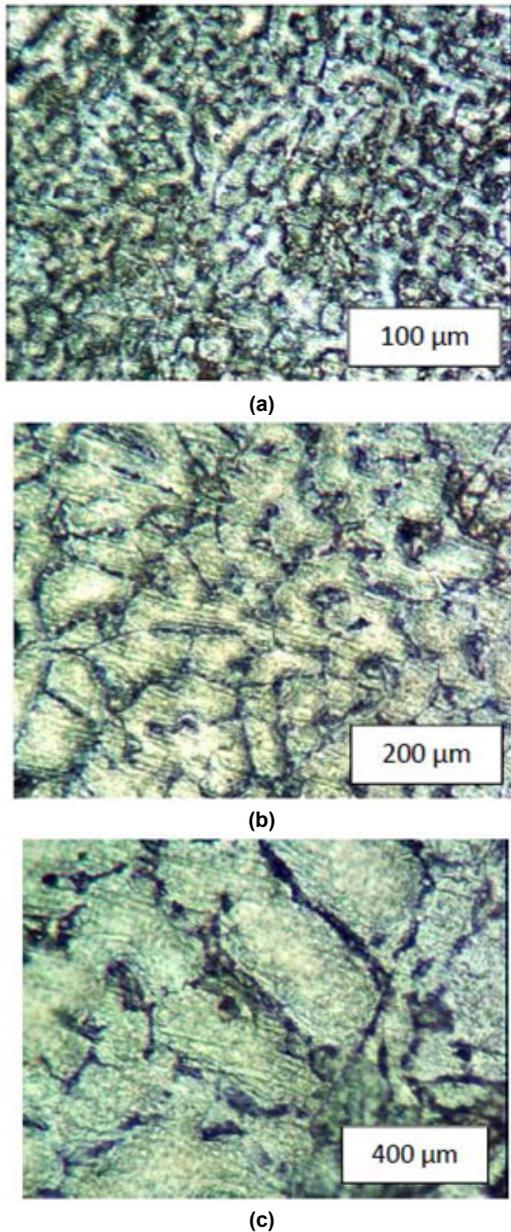
Figure 6 Optical microstructure of the aluminium alloy LM25 with 4 % Gr, (a) 100x (b) 200x and (c) 400x
