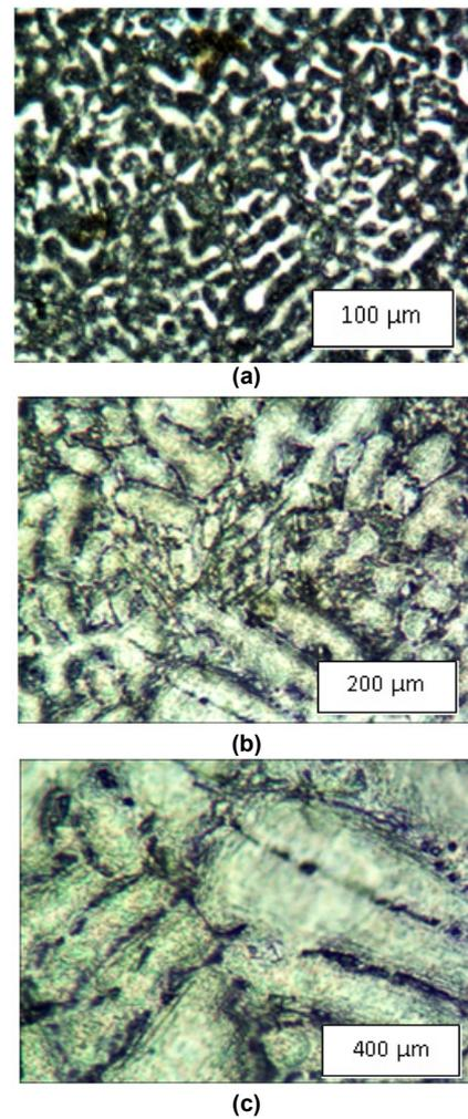
Figure 7. Optical microstructure of the aluminium alloy LM25 with 4 % Gr and 3 % of  $Fe_3O_4$ , (a) 100x (b) 200x and (c) 400x
