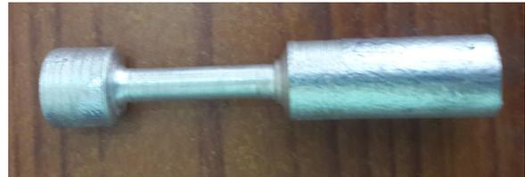
Figure 4 Dimension of tensile test specimen
