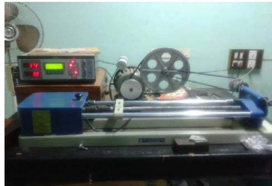
Figure 5 Micro Tensile Test - Digital tensometer
