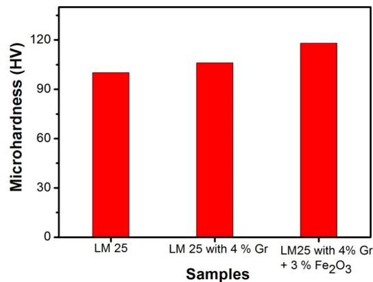
Figure 8. Microhardness result: A 200 grams load was utilized to produce an impression over the surface of the material for the dwell time of 20 seconds. From this hardness test, the value of microhardness for the sample such as LM25 alloy without reinforcement and the wt. % variation of different reinforcements such as Gr and  $Fe_3O_4$  in Al alloy MMCs were determined and it displayed shown in Figure 8.
