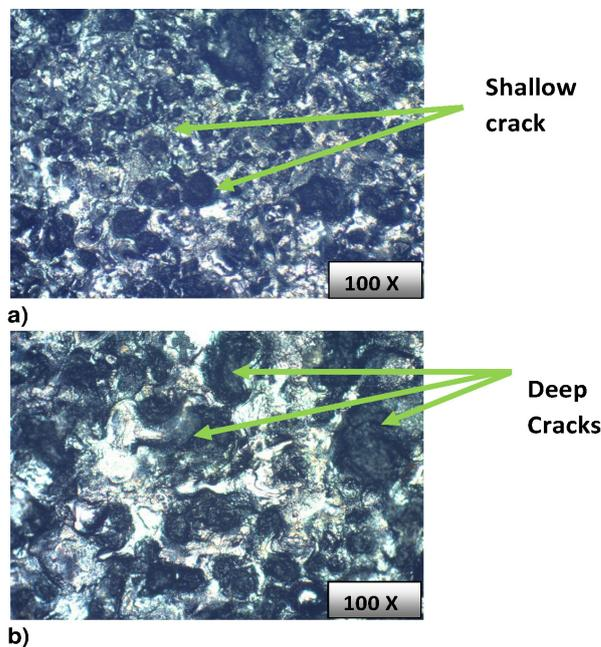
**Figure 5. Optical Micrograph of a) PMEDMed surface and b) Conventional EDMed surface**
