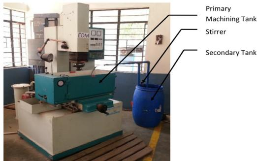
Figure 1. PMEDM set-up
