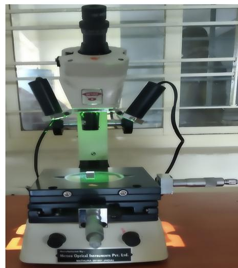
**Figure 5. Kerf taper measurement by Tool Makers Microscope**
