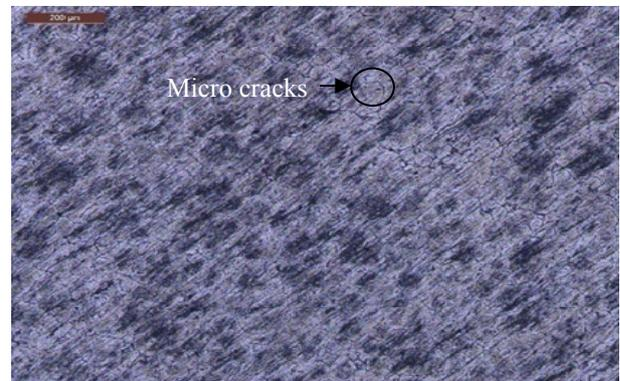
**Figure 9. Optical microscope image of specimen machined with TS-40mm/min, AFR-100gm/min, SOD-4mm detail of micro cracks**
