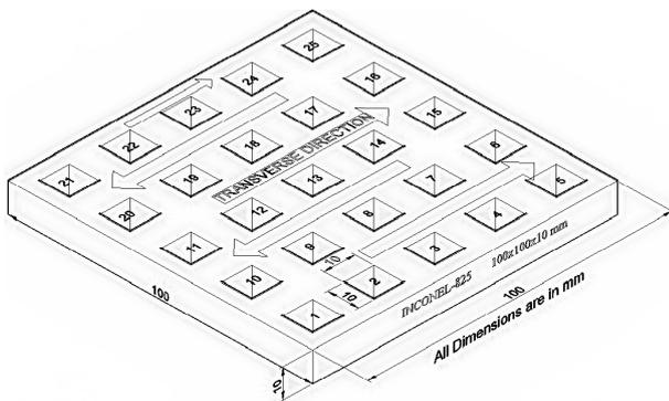
Figure 1. Inconel-825 Work piece Specimen
