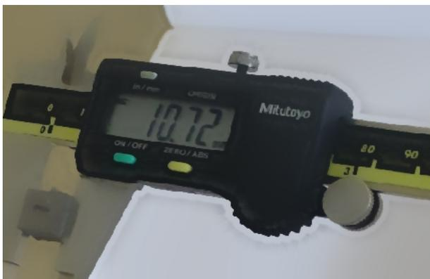
**Figure 4. Kerf width measurement by Vernier callipers**
