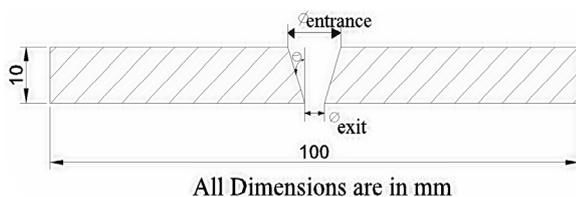
Figure 3. Kerf Taper geometry of an AWJM
