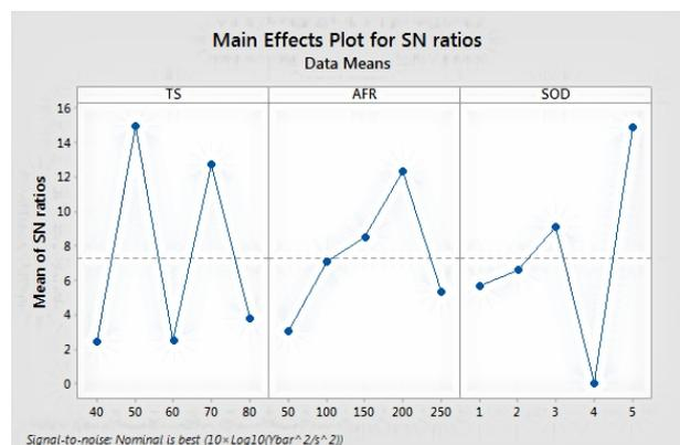
Figure 8. Main effect plot S/N Ratio for Over all Grey Relational grade.
