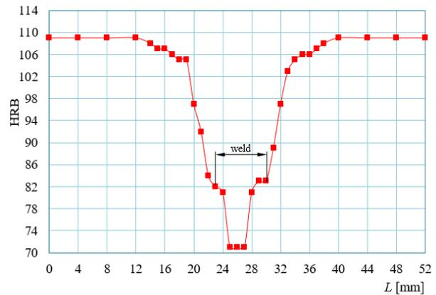
**Figure 4. Distribution of hardness over the surface of 1460 welded joints produced by TIG welding**
