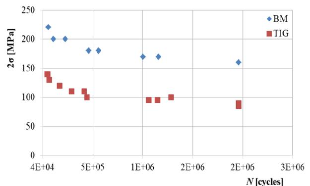
**Figure 6. S-N curves of base metal and TIG welded joints of 1460T1 aluminium alloy at stress ratio R = 0.1**
