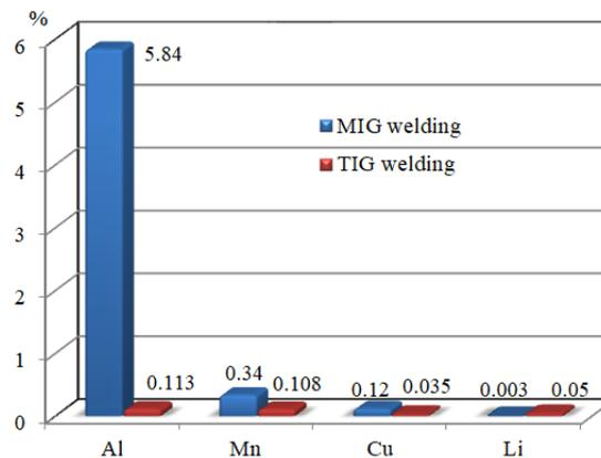
**Figure 2. Weight fraction of the main harmful SCWF during MIG and TIG welding of 1460 aluminium alloy**
