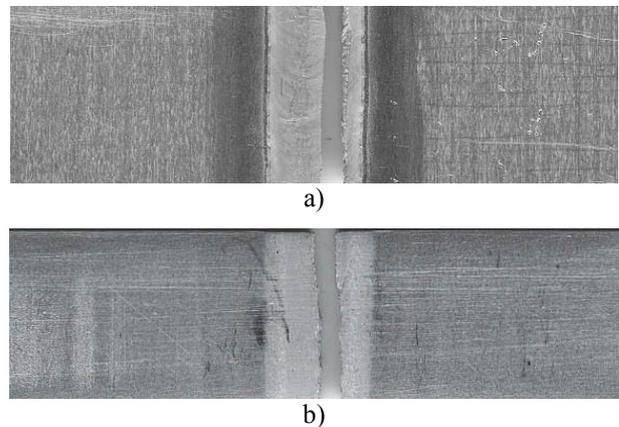
**Figure 5. Fragments of specimens of welded joints produced by TIG after tensile loading: a) with reinforcement, b) without reinforcement**
