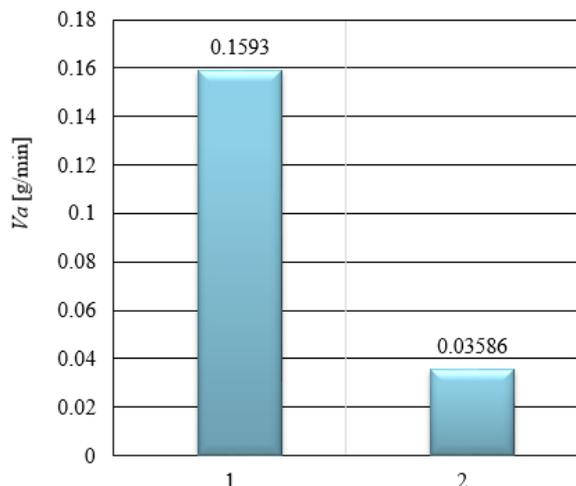
**Figure 1. Intensity of welding fume formation during MIG (1) and TIG (2) welding of 1460 aluminium alloy**
