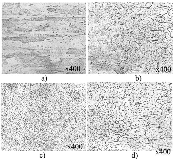
**Figure 3. Microstructure of welded joints of 1460 alloy produced by TIG welding using Sv1201 filler wire: a) base metal, b) and d) base metal fusion zones, c) weld metal**
