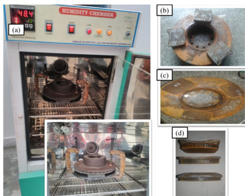
**Figure 2. Brake pad and rotor assembly for stiction test placed in the humidity chamber.**
