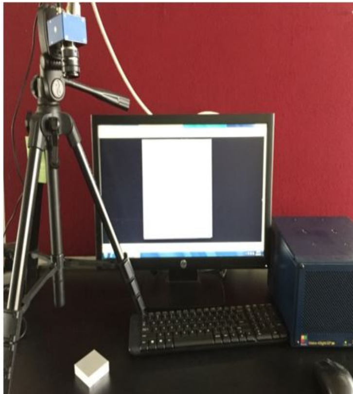
Fig. 3. Experimental setup to capture texture images through CCD
