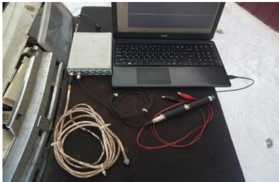
**Figure 8. Vibration instrumentation, a pressure sensor and an accelerometer**
