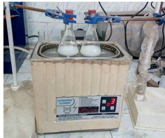
Figure 2. Preparation of Al 2 O 3 nanoparticles based fluid using ultrasonication technique.
