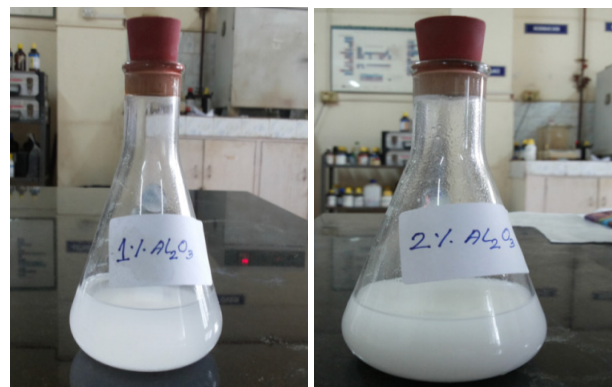
Figure 2. Preparation of Al 2 O 3 nanoparticles based fluid using ultrasonication technique.
